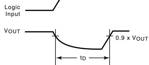
Figure 3. Break Before Make Interval Timing
