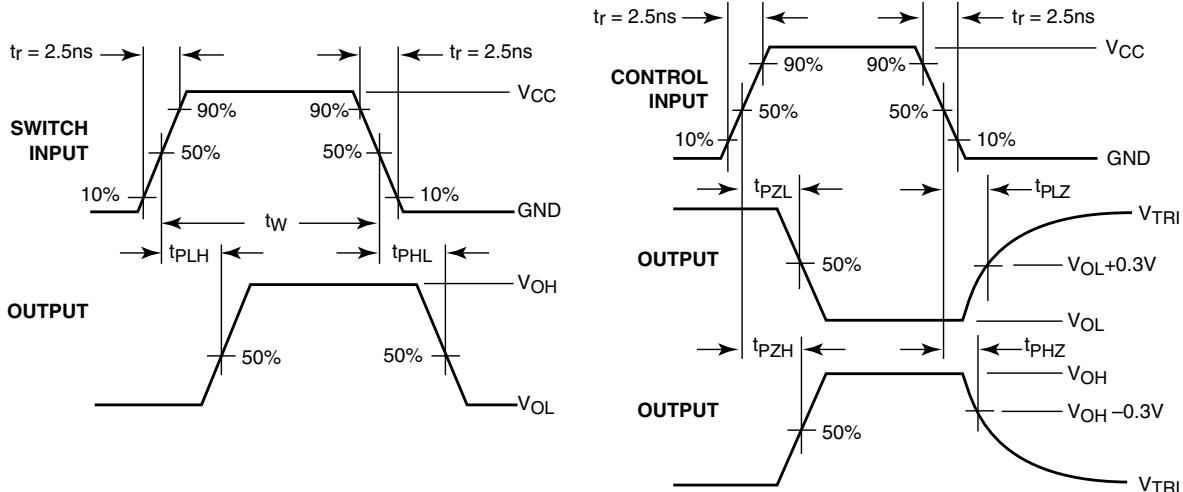
Figure 2. AC Waveforms
