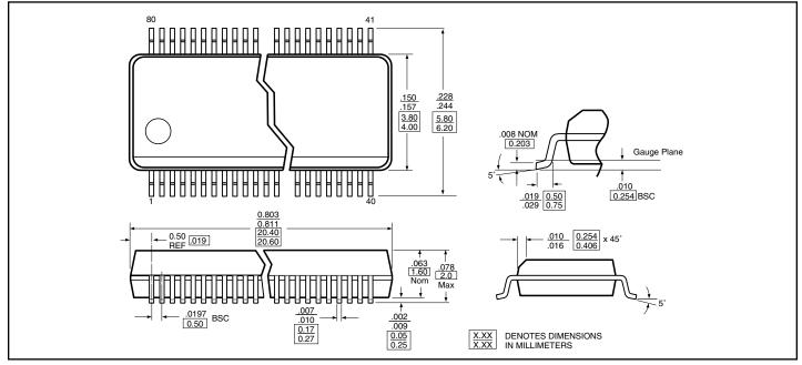
Packaging Mechanical: 80-Pin, Plastic Very Fine Pitch Dual Flat No-lead DFN (ZA)
