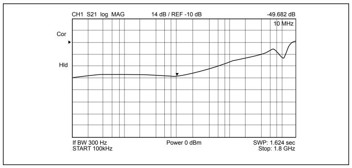
Figure 2. Off Isolation vs Frequency
