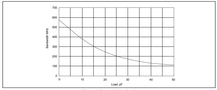
Figure 6. Bandwidth vs Load
