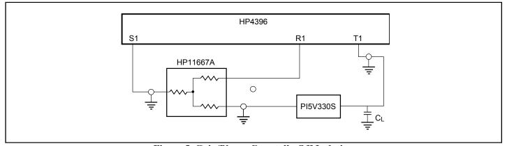
Figure 5. Gain/Phase, Crosstalk, Off-Isolation
