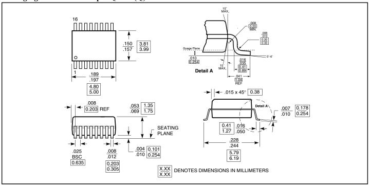
Packaging Mechanical: 16-pin SOIC (W)
