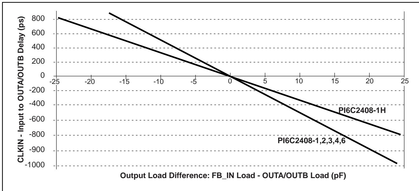
The relationship between loading of the FB\_IN signal and other outputs determines the input-output delay. Zero delay is achieved when all outputs, including feedback, are loaded equally.
