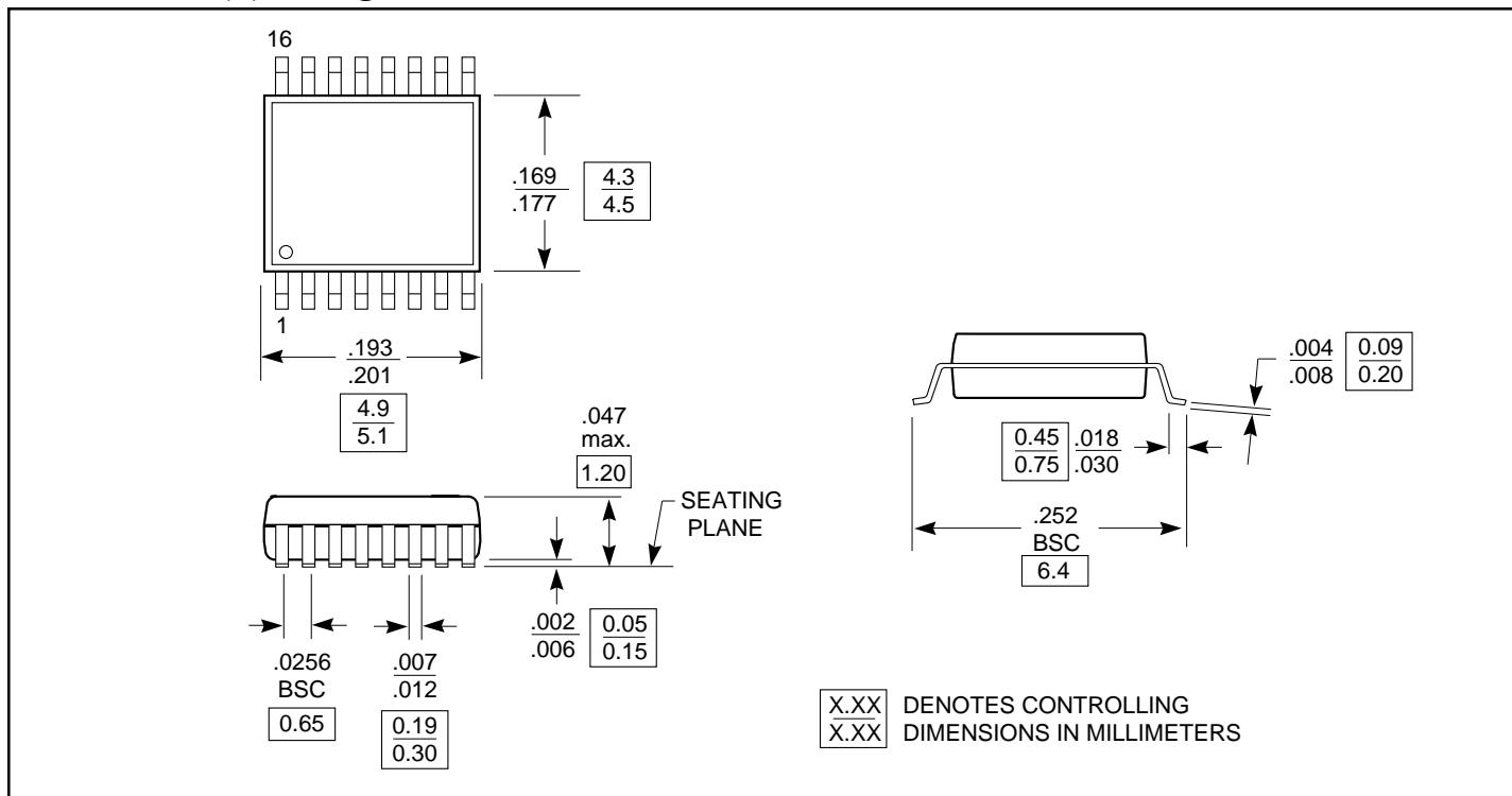
**Note:** Controlling dimensions in millimeters. Ref: JEDEC MS-012 AC
