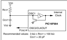
In RCIO mode, the RC circuit is connected to the OSC1 pin. The OSC2 pin becomes an additional general purpose I/O pin. The I/O pin becomes bit 4 of PORTA (RA4). Figure 3-6 shows the RCIO mode connections.
