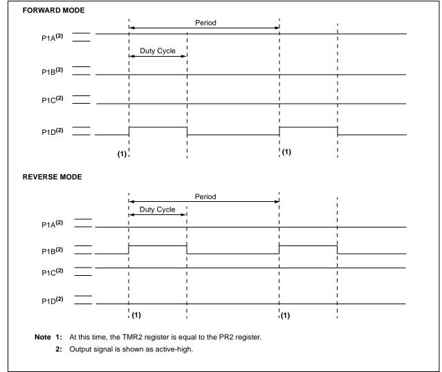
FIGURE 11-8: FULL-BRIDGE PWM OUTPUT
