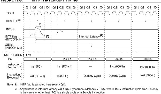
FIGURE 12-8: INT PIN INTERRUPT TIMING
