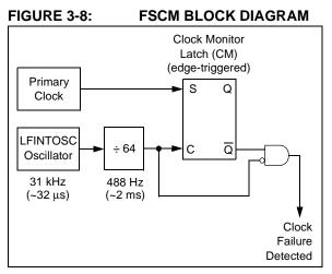
The FSCM function is enabled by setting the FCMEN bit in the Configuration Word register (CONFIG). It is applicable to all external clock options (LP, XT, HS, EC, RC or IO modes).
