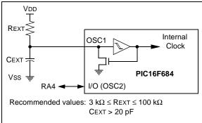
The RC oscillator frequency is a function of the supply voltage, the resistor (REXT) and capacitor (CEXT) values and the operating temperature. Other factors affecting the oscillator frequency are:
