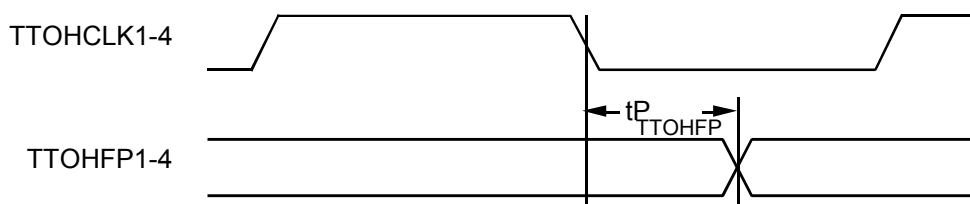
Figure 65 Transmit Overhead Output Timing
