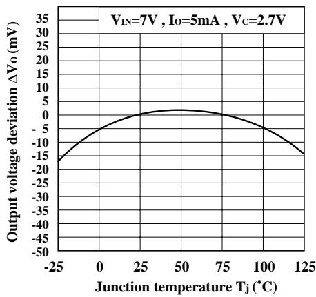
**Fig.7 Output Voltage Deviation vs. Junction Temperature (PQ12TZ51/11)**
