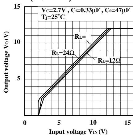
**Fig.10 Output Voltage vs. Input Voltage (Typical Value) (PQ12TZ51)**
