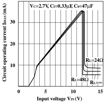
**Fig.20** Circuit Operating Current vs. Input Voltage (PQ09TZ11)
