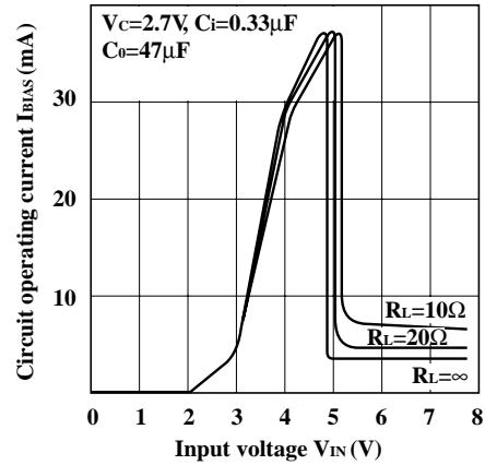
**Fig.18** Circuit Operating Current vs. Input Voltage (PQ12TZ51)
