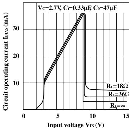
**Fig.19** Circuit Operating Current vs. Input Voltage (PQ05TZ11)
