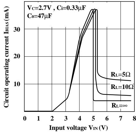
**Fig.16** Circuit Operating Current vs. Input Voltage (PQ05TZ51)
