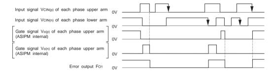
Note: Input interlock protection circuit; It is operated when the input signals for any upper-arm / lower-arm pair of a phase are simultaneously in "LOW" level.
