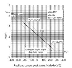
Fig. 5 OUTPUT CURRENT ANALOGUE SIGNALING "DATA HOLD" DEFINITION
