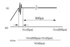
Note; Ringing happens around the point where the signal output voltage changes state from "analogue" to "data hold" due to test circuit arrangement and instrumentational trouble. Therefore, the rate of change is measured at a 5 µs delayed point.
