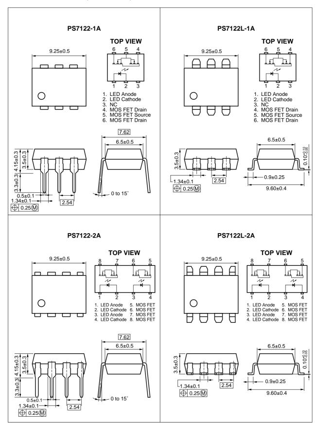
**PACKAGE DIMENSIONS (in millimeters)**
