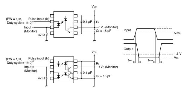
Remark C<sub>L</sub> is approximately 15 pF which includes probe and stray wiring capacitance.
