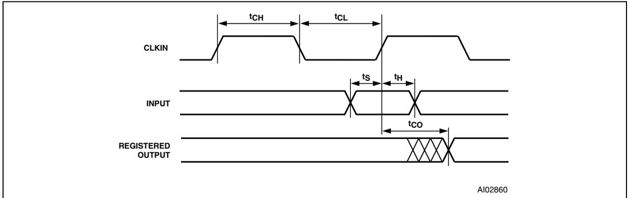
Table 49. CPLD Macrocell Synchronous Clock Mode Timing (5V devices)
