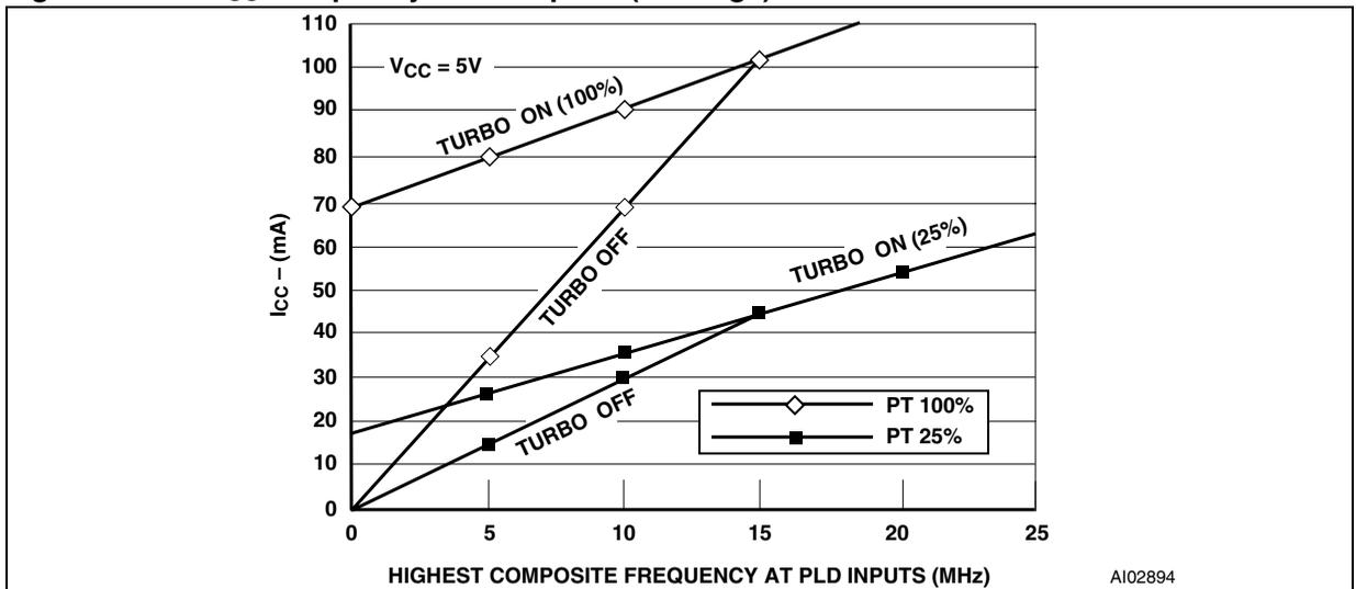
Figure 36. PLD I<sub>CC</sub> /Frequency Consumption (3V range)
