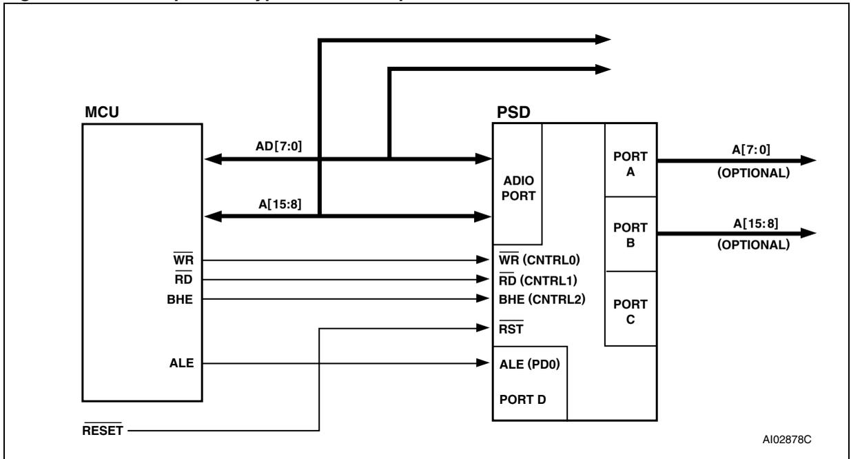
**PSD Interface to a Non-Multiplexed 8-Bit Bus**
