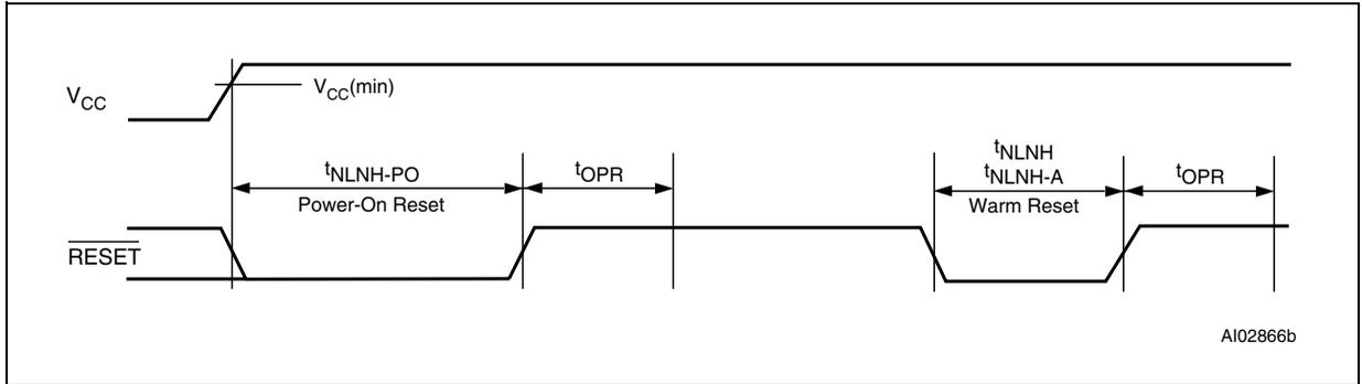
**Table 65. Reset ( $\overline{RESET}$ ) Timing (5V devices)**
