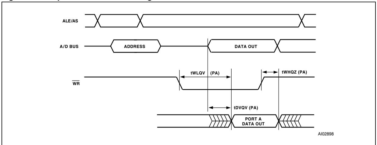
**Table 63. Port A Peripheral Data Mode WRITE Timing (5V devices)**
