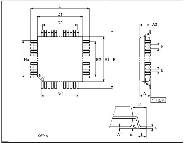
Figure 53. TQFP64 - 64-lead Thin Quad Flatpack, Package Outline
