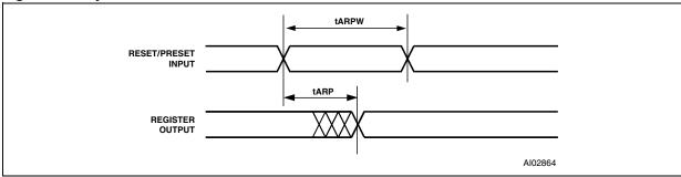
Figure 43. Asynchronous Clock Mode Timing (product term clock)
