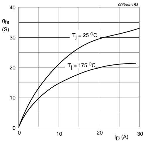
$T_j = 25 \text{ }^{\circ}C; V_{DS} > I_D \times R_{DSon}$
