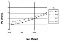
Note 1: All data listed in the above graphs, except for derating data, has been developed from actual products tested at 25°C. This data is considered typical data for the DC-DC Converter. Note 2: Thermal derating graphs are developed in free air convection cooling of 40-60 LFM.
