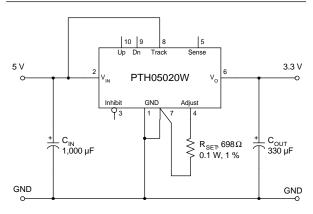
When the *Track* pin is connected to the input voltage the Auto-Track function is permanently disengaged. This allows the module to power up entirely under the control of its internal soft-start circuitry. When power up is under soft-start control, the output voltage rises to the set-point at a quicker and more linear rate.
