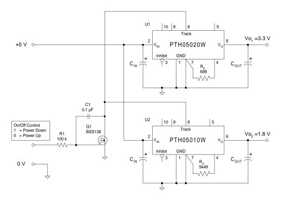
Figure 3-6; Simultaneous Power Up with Auto-Track Control
