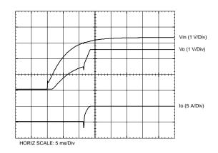
Figure 3-9; Application Circuit Demonstrating Pre-Bias Startup
