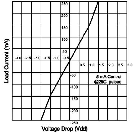
Figure 2. Linearity Characteristics
