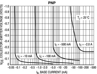
Figure 6. Collector Saturation Region
