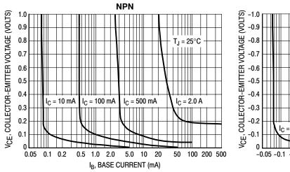
Figure 5. Collector Saturation Region
