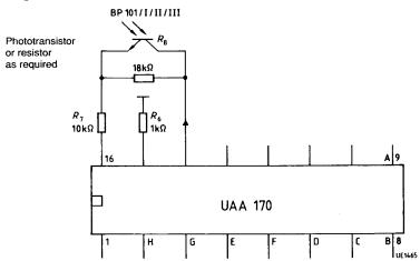
Pins 14, 15, and 16 serve to determine the diode current. Corresponding to the desired light intensity, the forward current of the diodes is linearly variable in the range  $I_1$  approx. 0 to 50 mA. The resistance at pin 15 defines the adjusting range. The resistances between pin 14 and 16 determine the current.
