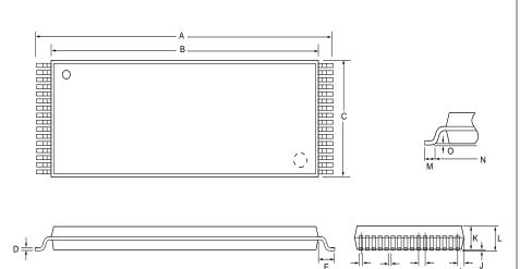
NOTE: Each lead certerline is located within .25mm[.01 inch] of its true position [TP] at a maximum at maximum material condition.
