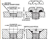
To assure maximum sealing performance of SEELSKREWS® and SEELBOLTS® a clearance hole must be used.
