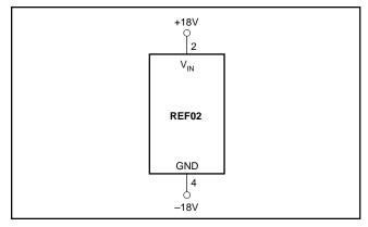
FIGURE 1. Burn-In Circuit.
