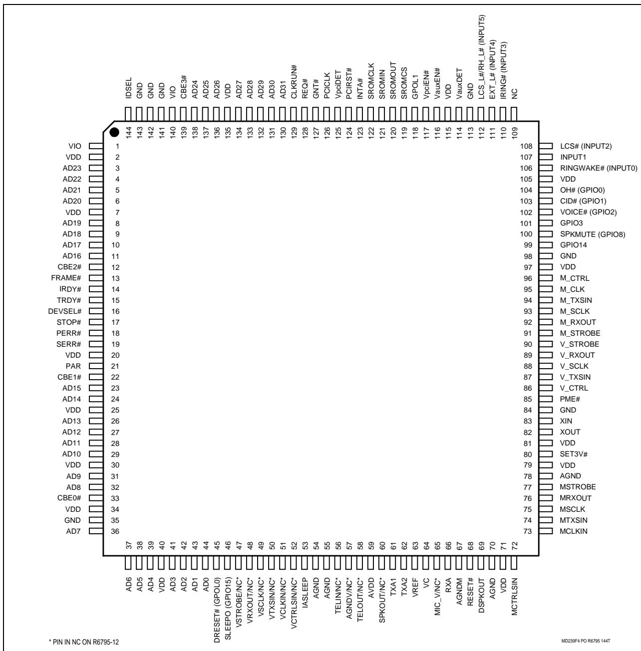
Figure 4. R6795 144-Pin TQFP Pin Signals
