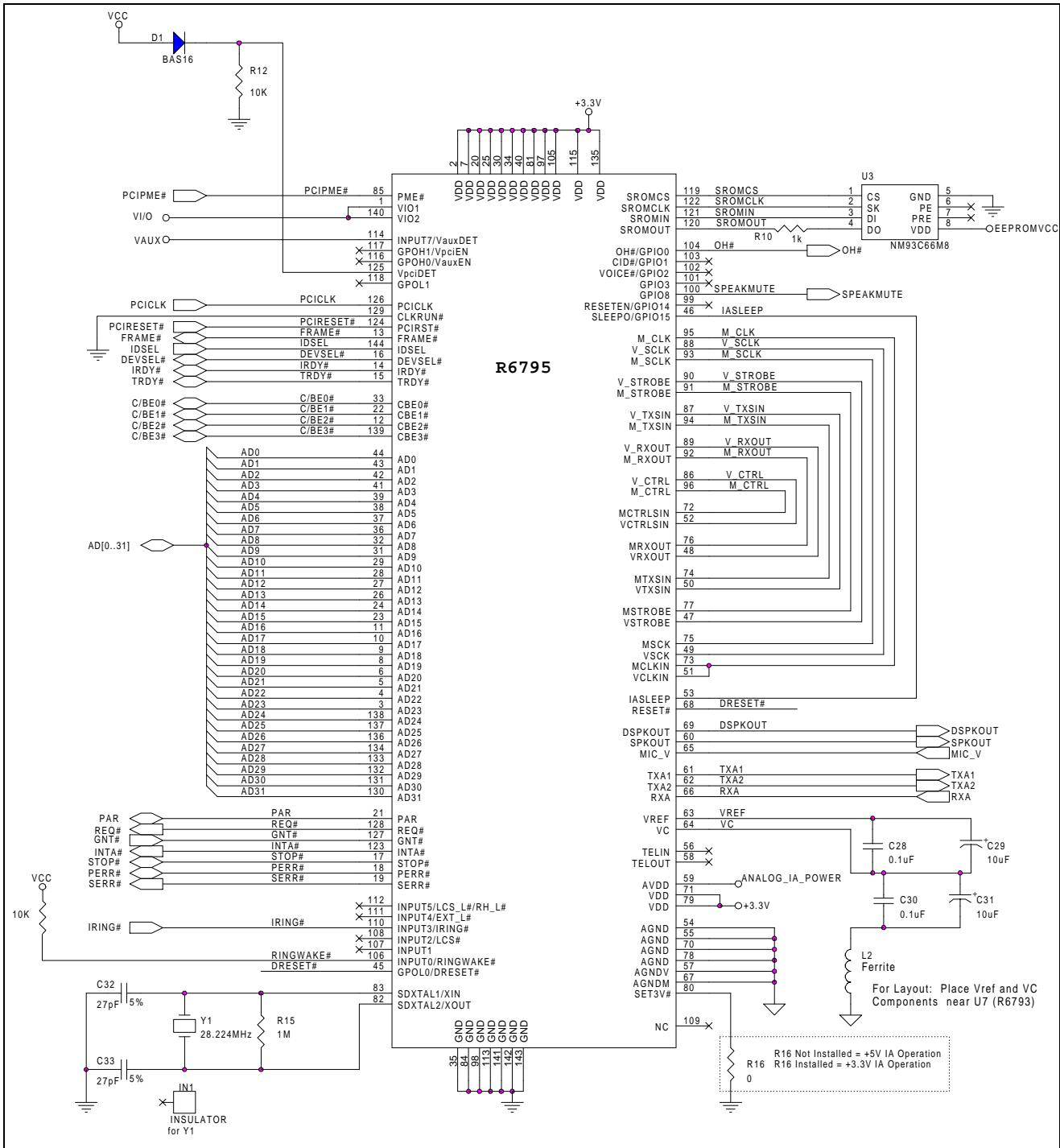
**Figure 5. Schematic - R6795 Interface –Speakerphone Application**
