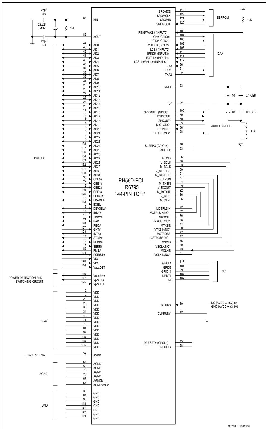
Figure 3. R6795 144-Pin TQFP Hardware Interface Signals
