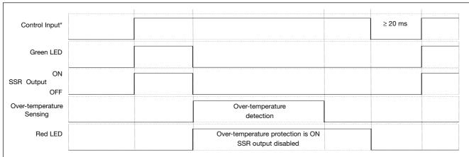
\*After over-temperature condition is removed, SSR can be reset by switching OFF the control input for more than 20 ms and switching back ON: this will switch ON the SSR output
