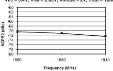
Low Power Mode (Vcc=1.4V, Vref=2.85V, Vmode=2V, Pout=16dBm)
