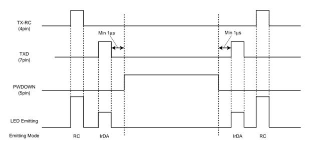
$* If TX-RC \ or \ TXD \ input \ pulse \ width \ is \ wider \ than \ 48 \mu s, \ output \ LED \ emitting \ pulse \ will \ be \ turn \ off \ approximately \ 48 \mu s.$
