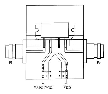
C : 10000pF,  $10\mu$ F PARALLEL L :  $\phi$ 0.5, 3ID, 5T ENAMEL WIRE
