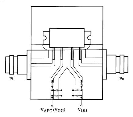
C : 10000pF,  $10\mu\text{F}$  PARALLEL L :  $\phi 0.5$ , 3ID, 5T ENAMEL WIRE
