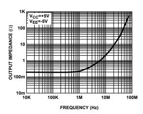
FIGURE 12. CLOSED LOOP OUTPUT IMPEDANCE
