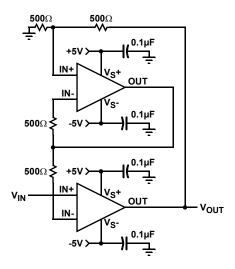
FIGURE 22. FAST-SETTLING PRECISION AMPLIFIER
