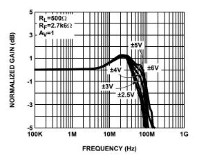
FIGURE 3. FREQUENCY RESPONSE FOR VARIOUS  $V_{CC}$ ,  $V_{EE}$
