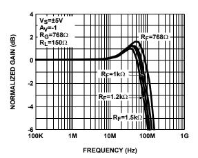
FIGURE 14. FREQUENCY RESPONSE FOR VARIOUS FEEDBACK RESISTORS, A<sub>V</sub>=-1
