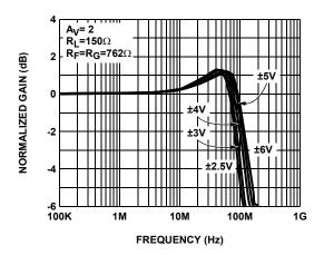
FIGURE 4. FREQUENCY RESPONSE FOR VARIOUS VCC, VEE
