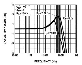
FIGURE 16. FREQUENCY RESPONSE FOR VARIOUS FEEDBACK RESISTORS, A<sub>V</sub>=+1
