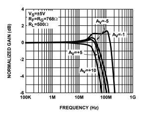
FIGURE 15. FREQUENCY RESPONSE FOR VARIOUS GAIN SETTINGS
