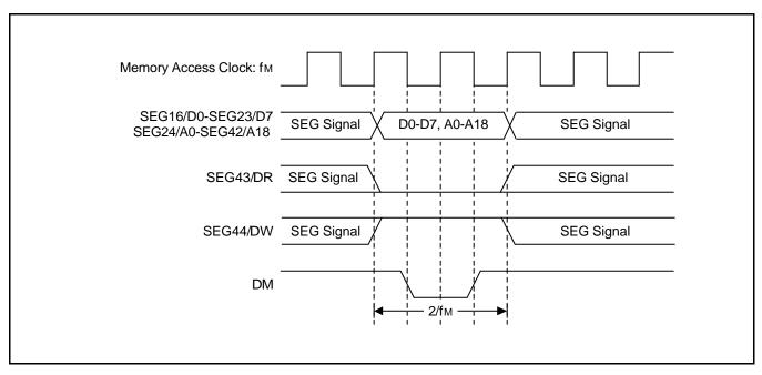
Figure 13-2. External Memory Read Cycle Timing Diagram
