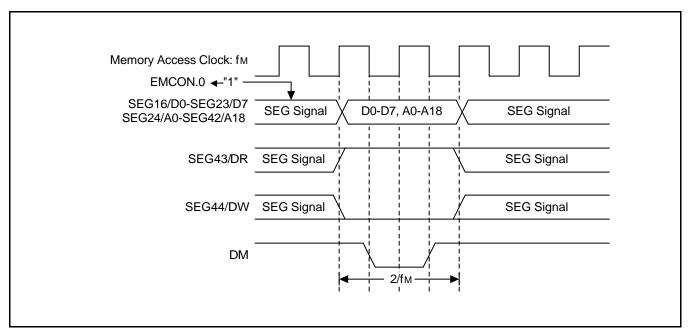
Figure 13-1. External Memory Write Cycle Timing Diagram
