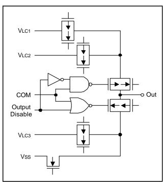
Figure 1-12. Pin Circuit Type H-7
