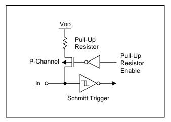
Figure 1-4. Pin Circuit Type A-3
