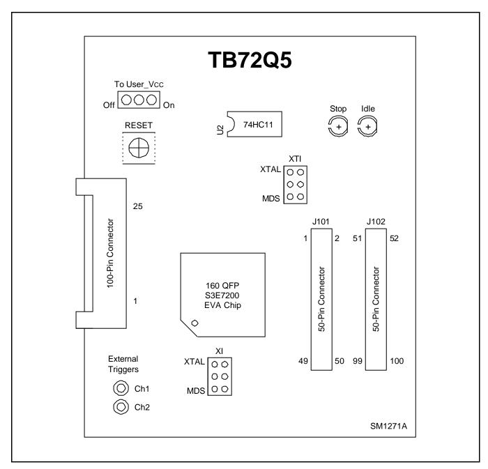
Figure 17-2. TB72Q5 Target Board Configuration
