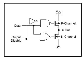
Figure 1-6. Pin Circuit Type C
