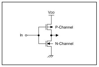
Figure 1-3. Pin Circuit Type A
