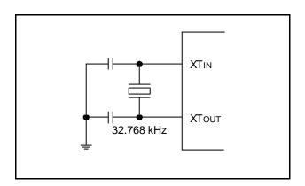
Figure 6-5. Crystal/Ceramic Oscillator
