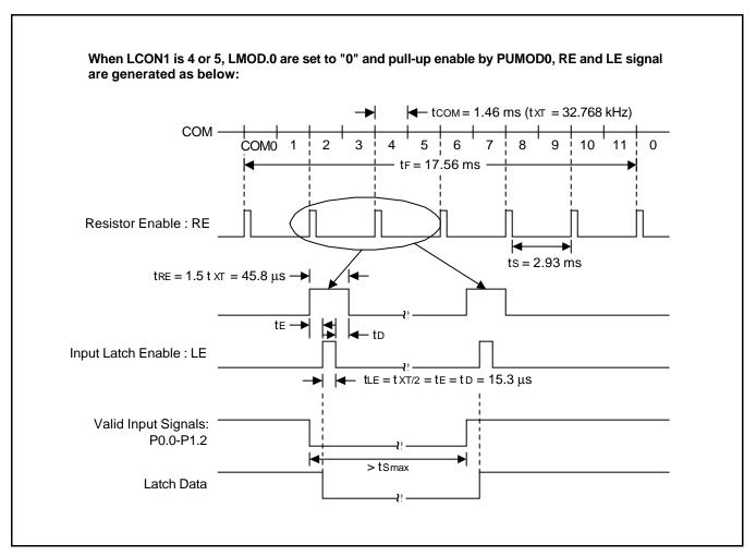
Figure 12-11. RE, LE and Inputs Signal Waveform (1/12 Duty)
