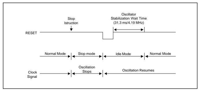
Figure 8-3. Timing When Stop Mode is Released by RESET
