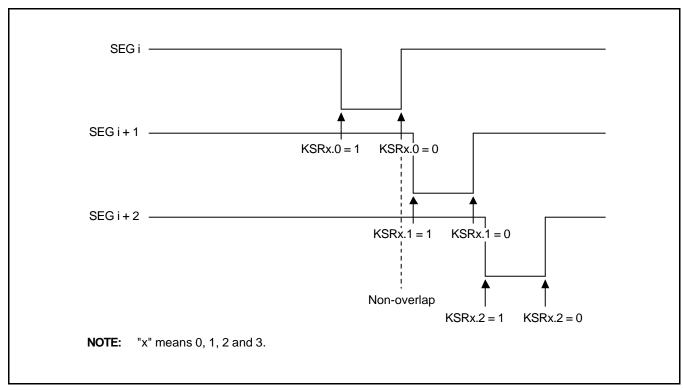
Figure 12-13. Segment Pin Output Signal When LCON1.3 = 1
