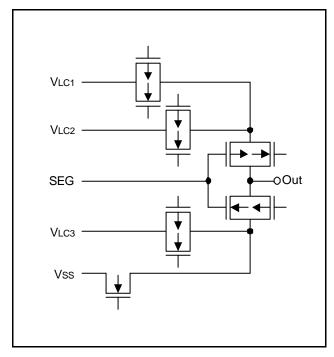
Figure 1-10. Pin Circuit Type H-5
