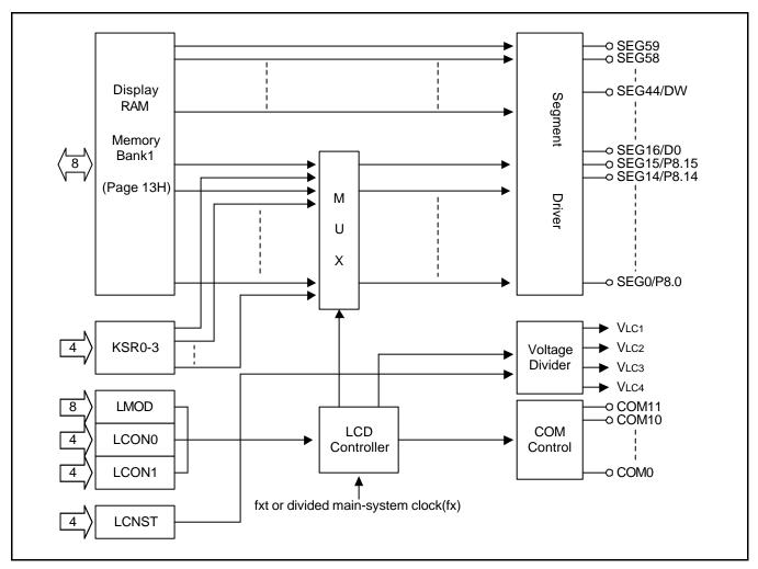
Figure 12-1. LCD Circuit Diagram
