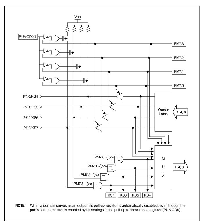
Figure 10-5. Port 7 Circuit Diagram
