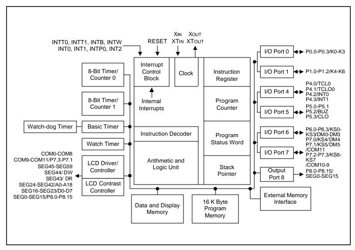
Figure 1-1. S3C72Q5/P72Q5 Specified Block Diagram
