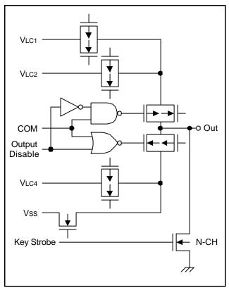
Figure 1-9. Pin Circuit Type H-4
