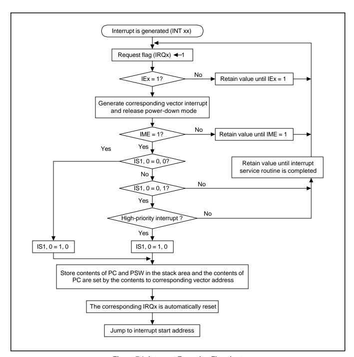
Figure 7-1. Interrupt Execution Flowchart
