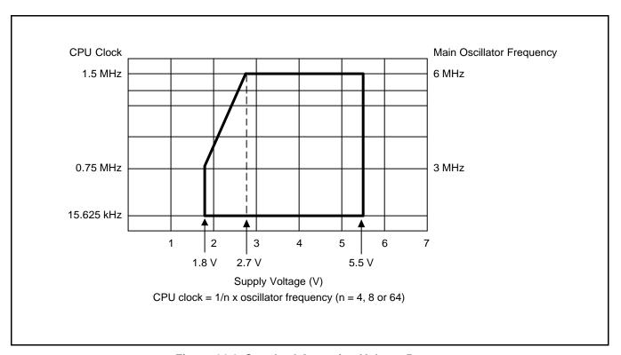
Figure 14-1. Standard Operating Voltage Range
