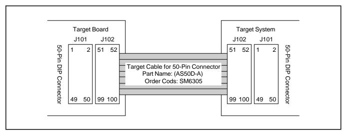
Figure 17-4. TB72Q5 Adapter Cable for 100-QFP Package (S3C72Q5/P72Q5)
