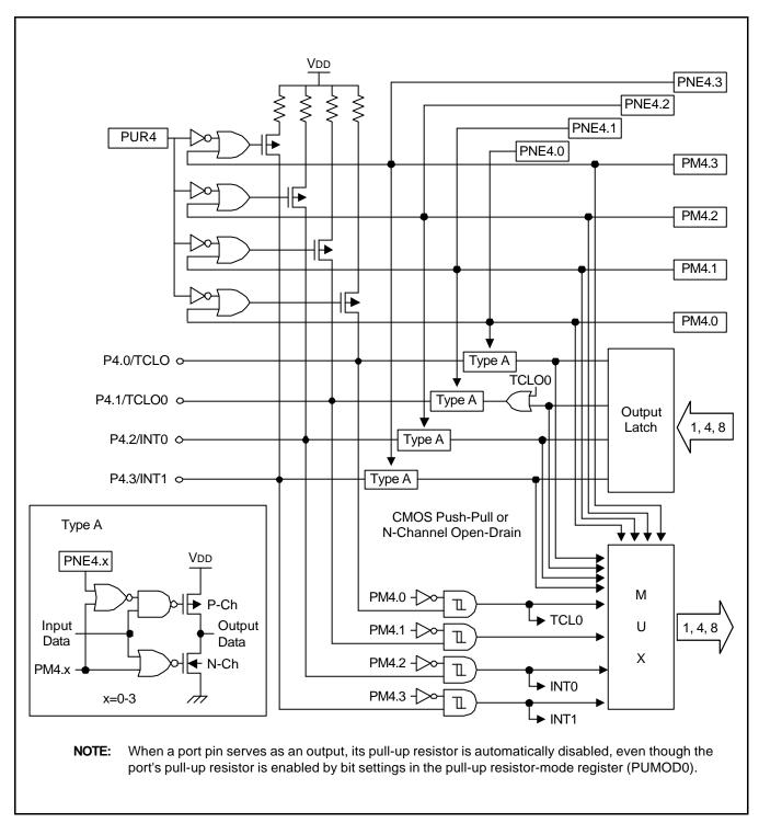
Figure 10-2. Port 4 Circuit Diagram
