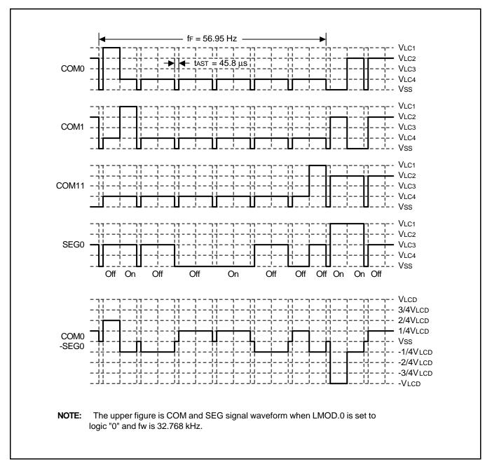
Figure 12-12. LCD Signal Waveform for 1/12 Duty and 1/4 Bias
