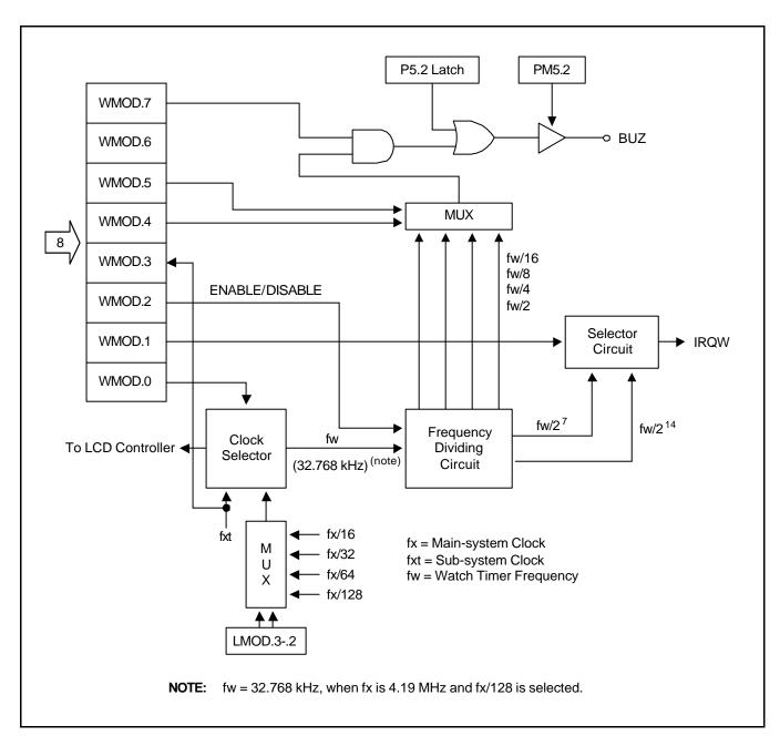
Figure 11-6. Watch Timer Circuit Diagram
