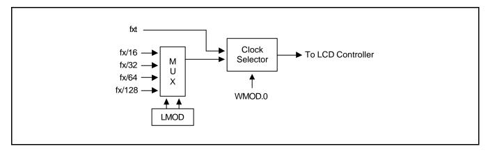
Figure 12-2. LCD Clock Circuit Diagram
