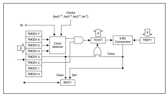
Figure 11-4. TC1 Circuit Diagram
