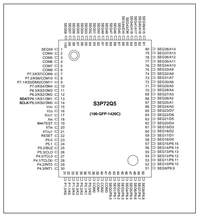
Figure 16-1. S3P72Q5 Pin Assignments (100-QFP Package)
