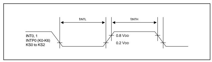
Figure 14-5. Input Timing for External Interrupts and Quasi-Interrupts
