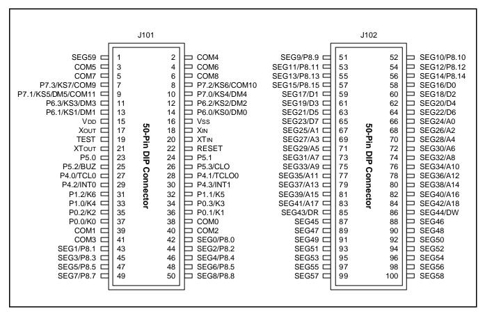
Figure 17-3. 50-Pin Connectors for TB72Q5
