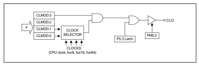
Figure 6-7. CLO Output Pin Circuit Diagram
