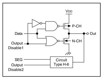
Figure 1-15. Pin Circuit Type H-11
