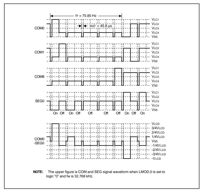
Figure 12-6. LCD Signal Waveform for 1/9 Duty and 1/4 Bias
