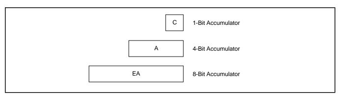
Figure 2-6. 1-Bit, 4-Bit, and 8-Bit Accumulator
