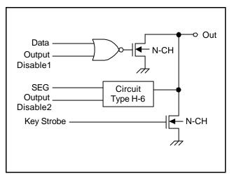
Figure 1-13. Pin Circuit Type H-9
