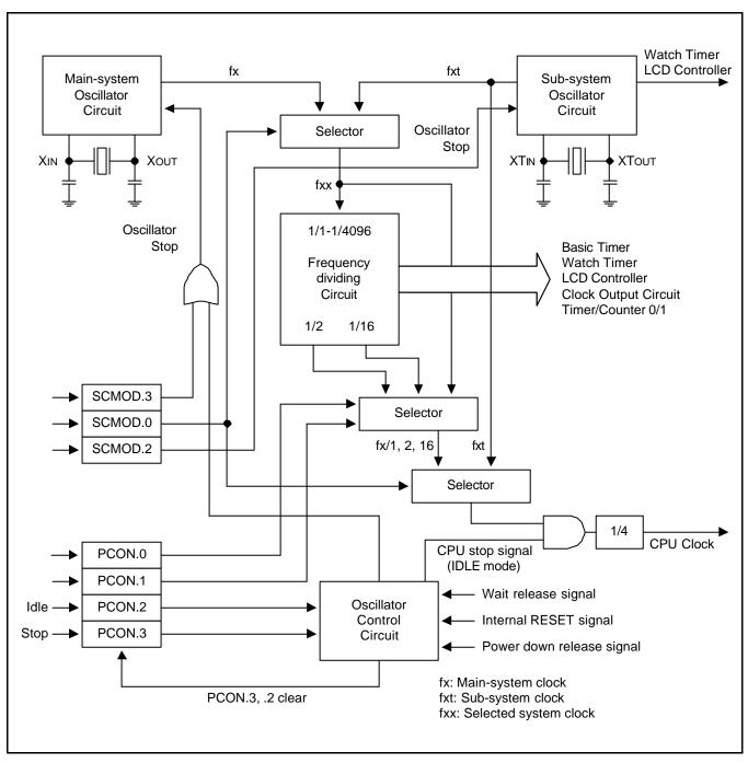
Figure 6-1. Clock Circuit Diagram
