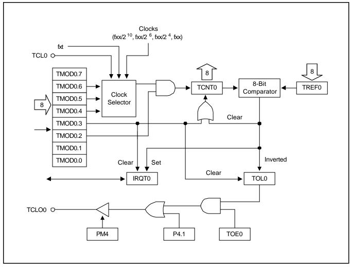
Figure 11-2. TC0 Circuit Diagram
