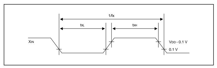
Figure 14-6. Clock Timing Measurement at  $X_{\text{IN}}$
