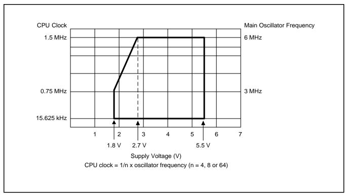
Figure 16-2. Standard Operating Voltage Range
