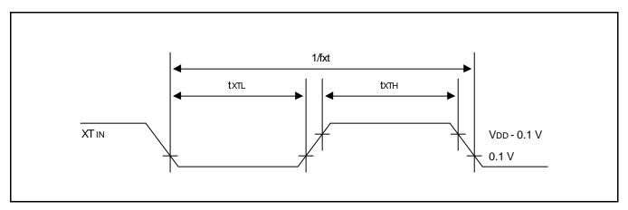
Figure 14-7. Clock Timing Measurement at  $\mathrm{XT}_{\mathrm{IN}}$
