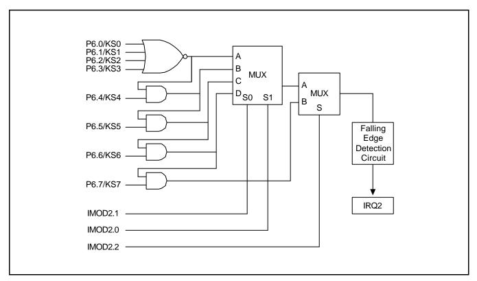
Figure 7-6. Circuit Diagram for INT2
