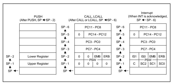
Figure 2-7. Push-Type Stack Operations
