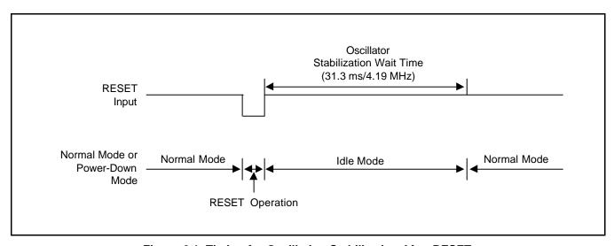
Figure 9-1. Timing for Oscillation Stabilization After RESET
