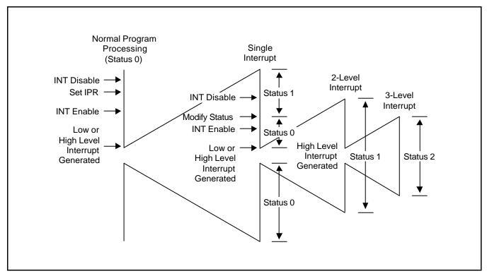
Figure 7-4. Multi-Level Interrupt Handling
