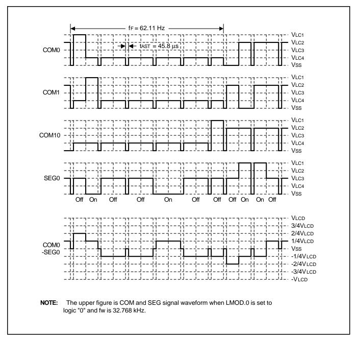
Figure 12-10. LCD Signal Waveform for 1/11 Duty and 1/4 Bias
