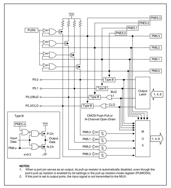
Figure 10-3. Port 5 Circuit Diagram
