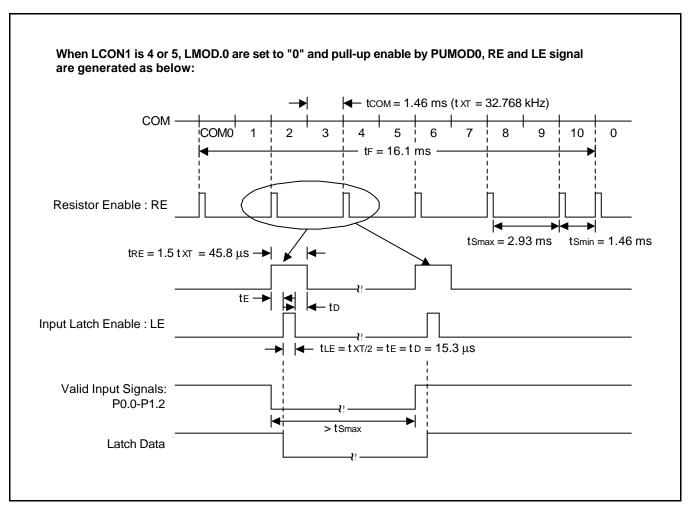
Figure 12-9. RE, LE and Inputs Signal Waveform (1/11 Duty)
