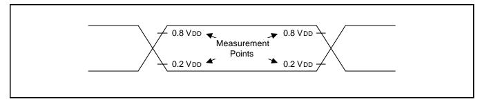
Figure 14-4. A.C. Timing Measurement Points (Except for X<sub>IN</sub> and XT<sub>IN</sub>)
