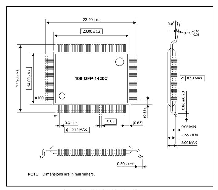
Figure 15-1. 100-QFP-1420 Package Dimensions
