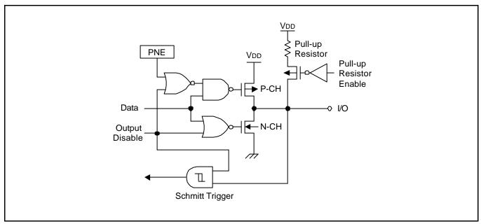
Figure 1-7. Pin Circuit Type E-2
