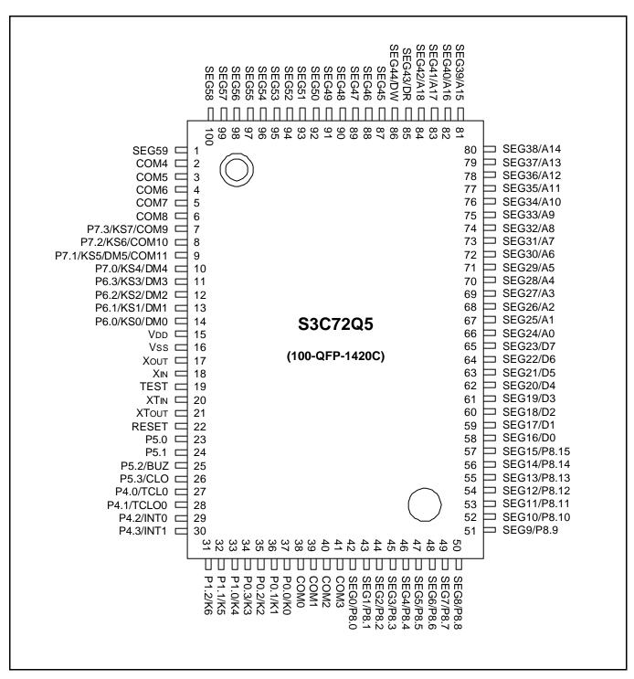
Figure 1-2. S3C72Q5 Pin Assignment Diagram
