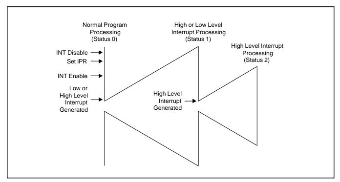
Figure 7-3. Two-Level Interrupt Handling
