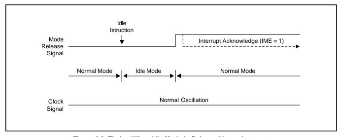
Figure 8-2. Timing When Idle Mode is Released by an Interrupt
