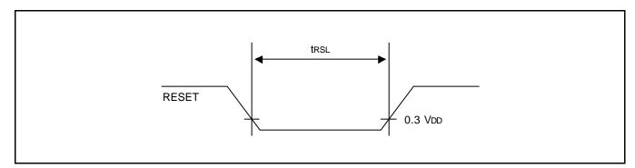
Figure 14-7. Input Timing for RESET Signal
