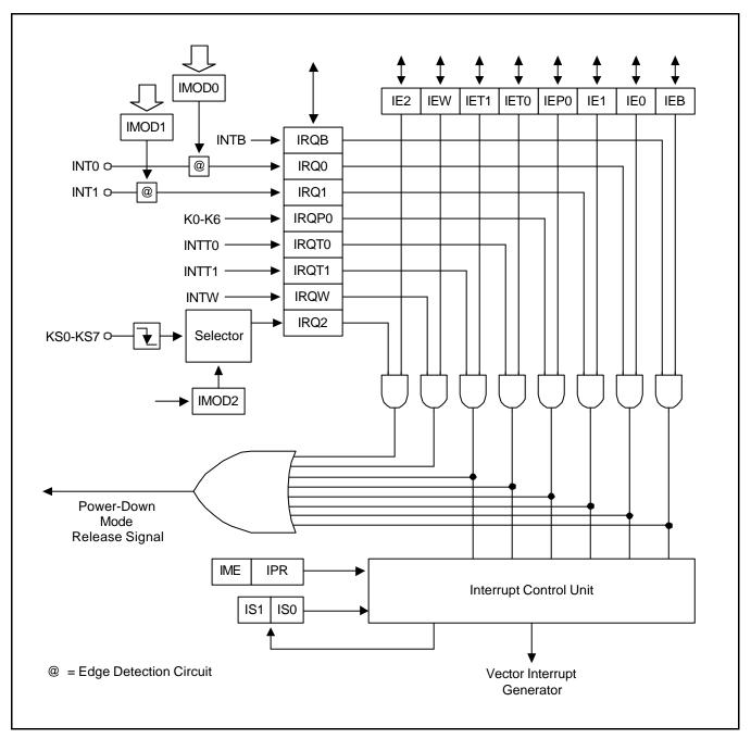
Figure 7-2. Interrupt Control Circuit Diagram
