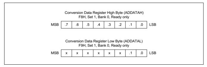
Figure 15-3. A/D Converter Data Register (ADDATAH/L)
