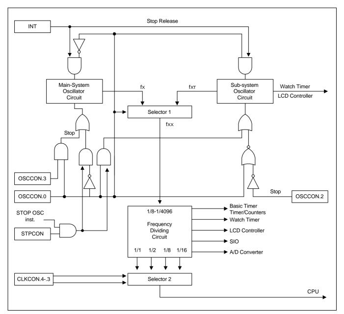
Figure 7-6. System Clock Circuit Diagram
