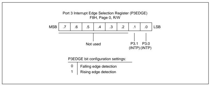
Figure 9-17. Port 3 Interrupt Edge Selection Register (P3EDGE)
