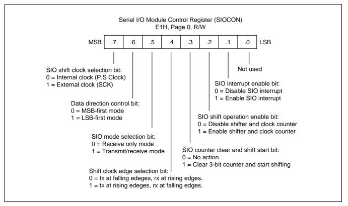
Figure 15-1. Serial I/O Module Control Register (SIOCON)
