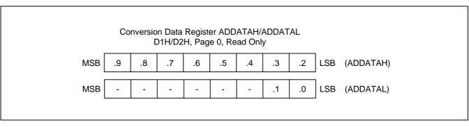
Figure 14-2. A/D Converter Data Register (ADDATAH/ADDATAL)
