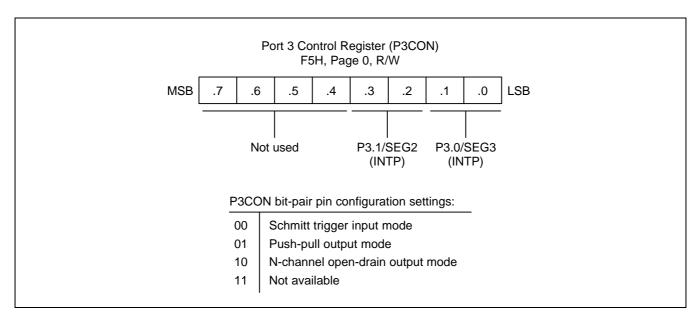
Figure 9-14. Port 3 Control Register (P3CON)
