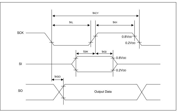
Figure 16-5. Serial Data Transfer Timing
