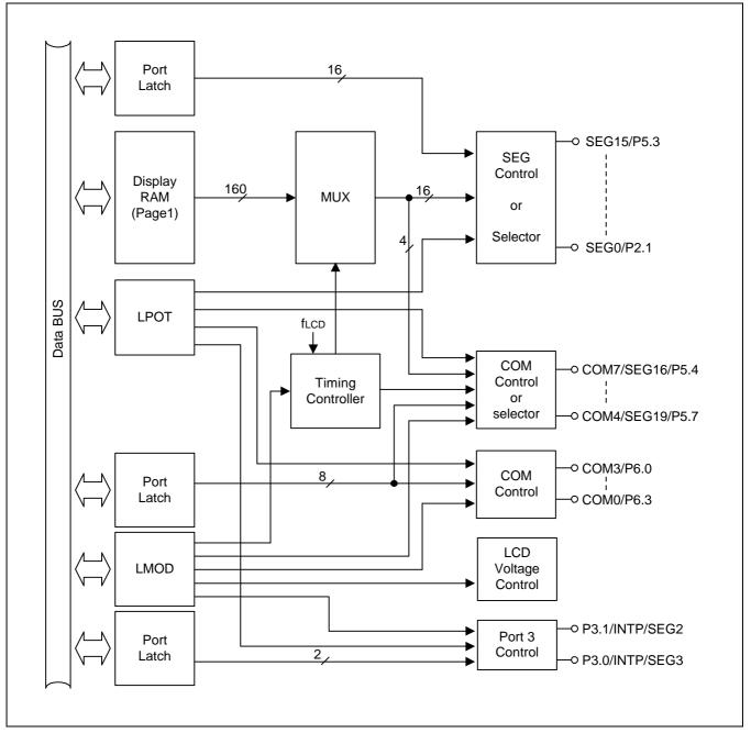
Figure 13-2. LCD Circuit Diagram
