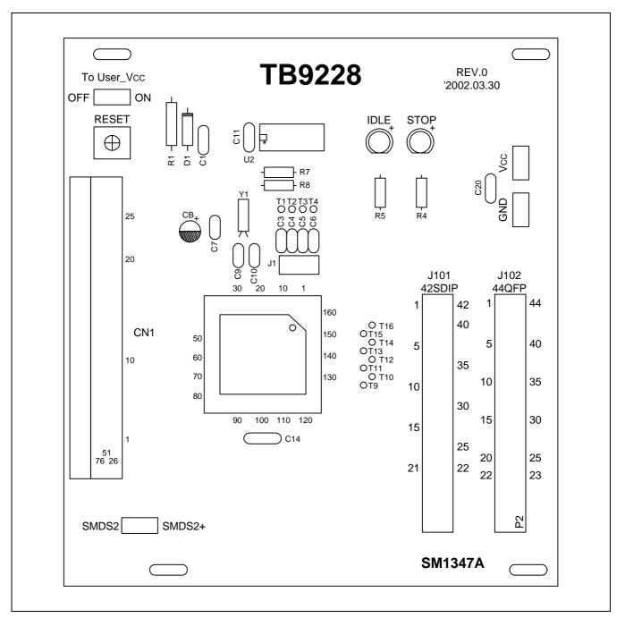
Figure 19-2. TB9228 Target Board Configuration
