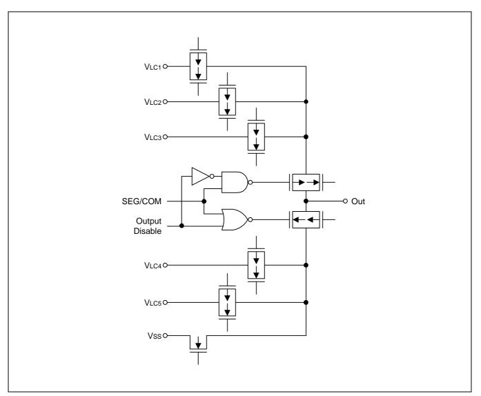
Figure 1-9. Pin Circuit Type H-23
