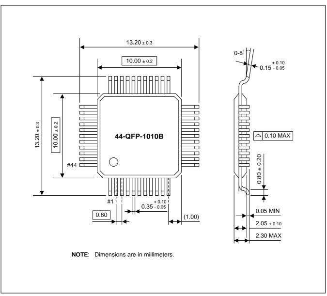
Figure 17-2. 44-QFP-1010B Package Dimensions
