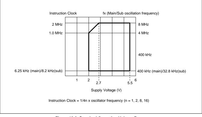
Figure 18-3. Standard Operating Voltage Range
