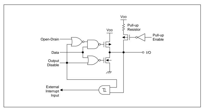
Figure 1-7. Pin Circuit Type E-4
