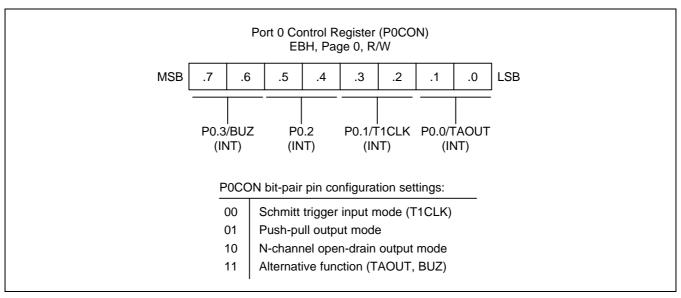
Figure 9-2. Port 0 Control Register (P0CON)
