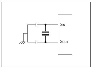
Figure 7-1. Crystal/Ceramic Oscillator
