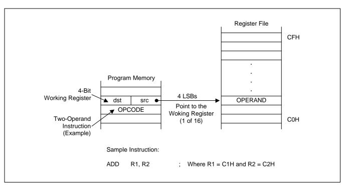
Figure 3-2. Working Register Addressing
