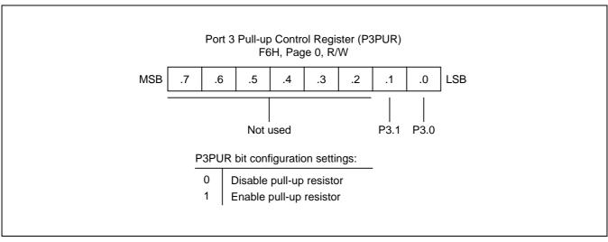
Figure 9-18. Port 3 Pull-up Control Register (P3PUR)
