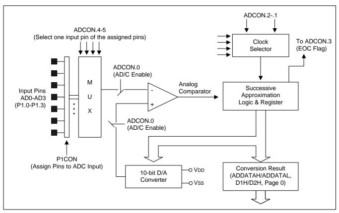
Figure 14-3. A/D Converter Functional Block Diagram
