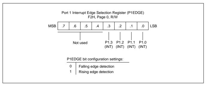
Figure 9-10. Port 1 Interrupt Edge Selection Register (P1EDGE)
