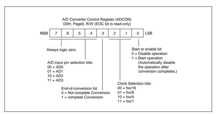
Figure 14-1. A/D Converter Control Register (ADCON)
