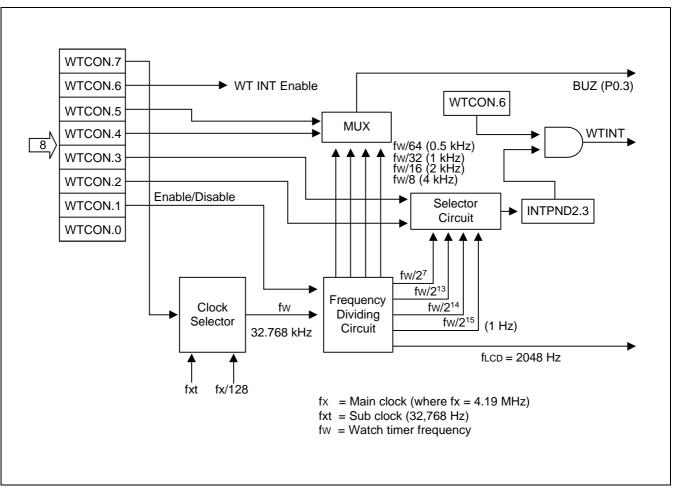
Figure 12-2. Watch Timer Circuit Diagram
