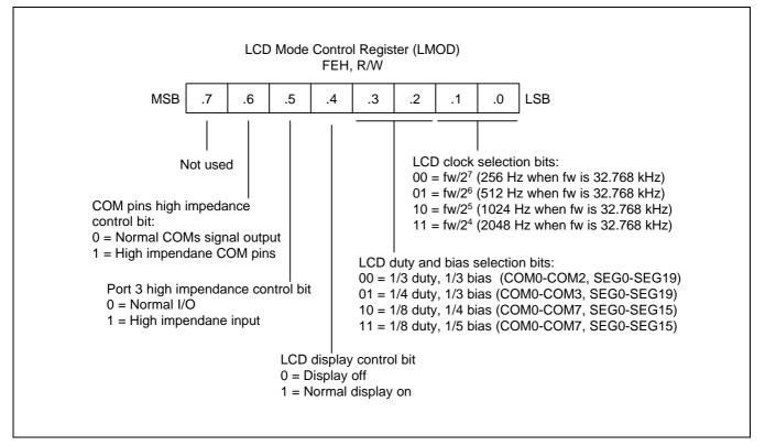
Figure 13-4. LCD Mode Control Register (LMOD)
