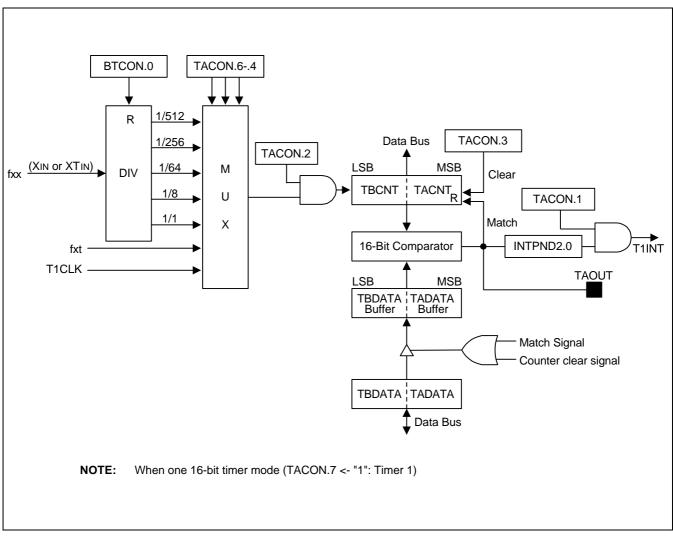
Figure 11-2. Timer 1 Block Diagram (One 16-bit Mode)
