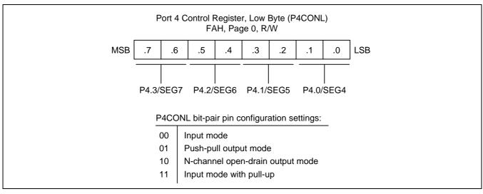
Figure 9-20. Port 4 Low-Byte Control Register (P4CONL)
