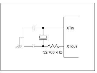
Figure 7-4. Crystal/Ceramic Oscillator
