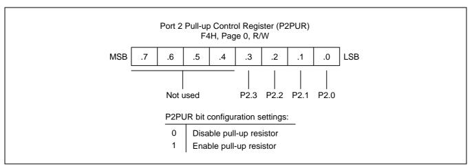
Figure 9-13. Port 2 Pull-up Control Register (P2PUR)
