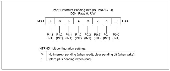
Figure 9-9. Port 1 Interrupt Pending Bits (INTPND1.7-.4)
