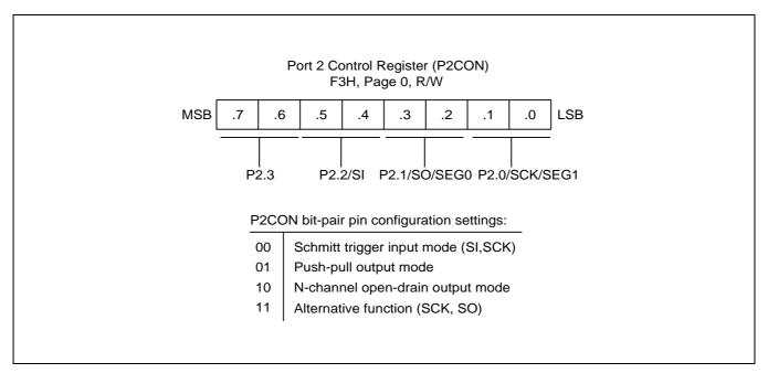
Figure 9-12. Port 2 Control Register (P2CON)
