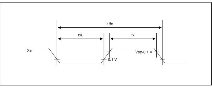
Figure 16-6. Clock Timing Measurement at X<sub>IN</sub>
