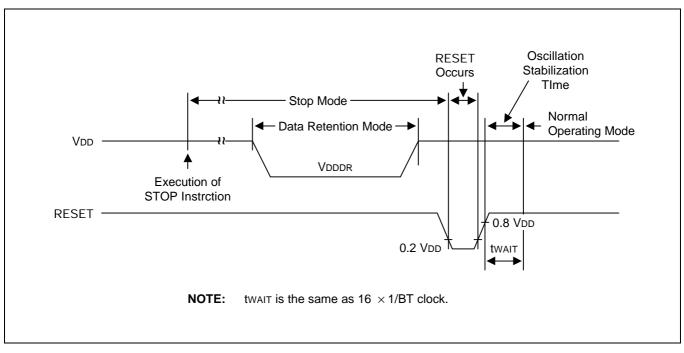
Figure 16-2. Stop Mode Release Timing When Initiated by a RESET
