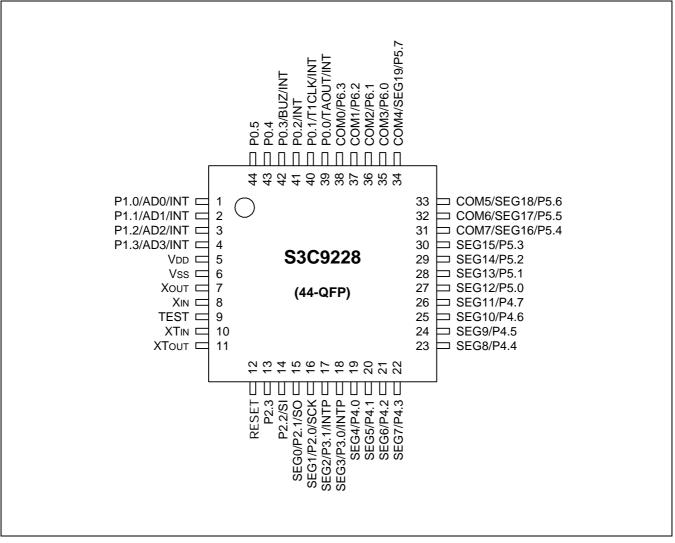
Figure 1-2. S3C9228 44-QFP Pin Assignments
