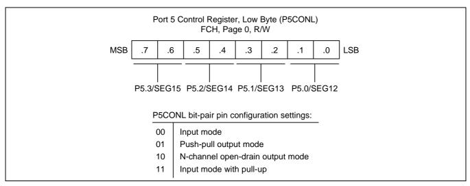
Figure 9-22. Port 5 Low-Byte Control Register (P5CONL)
