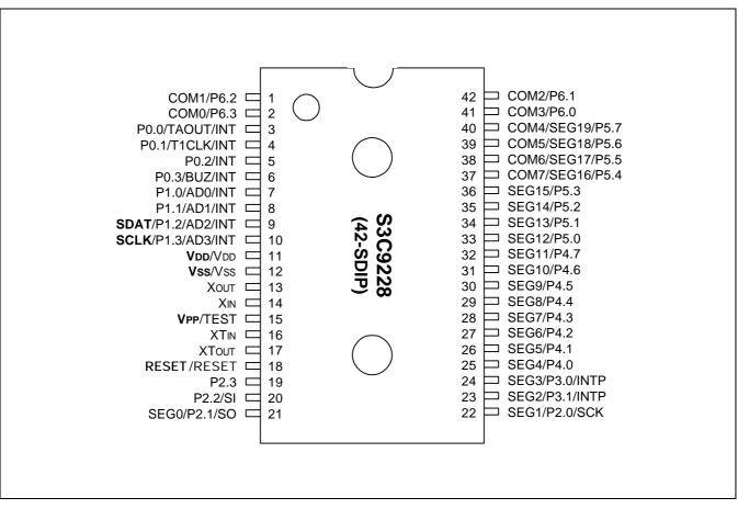
Figure 18-2. S3P9228 42-SDIP Pin Assignments
