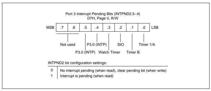
Figure 9-16. Port 3 Interrupt Pending Bits (INTPND2.5-.4)
