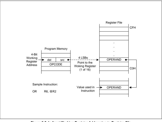
Figure 3-5. Indirect Working Register Addressing to Register File
