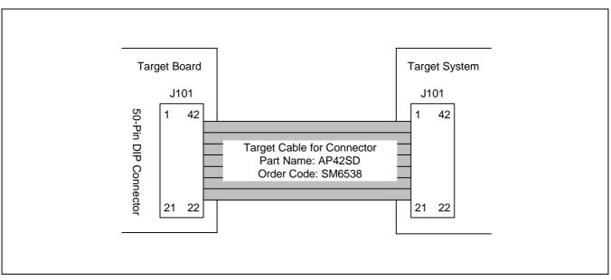
Figure 19-4. S3C9228 Probe Adapter for 42-SDIP Package
