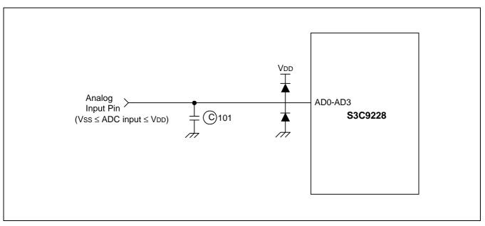
Figure 14-4. Recommended A/D Converter Circuit for Highest Absolute Accuracy
