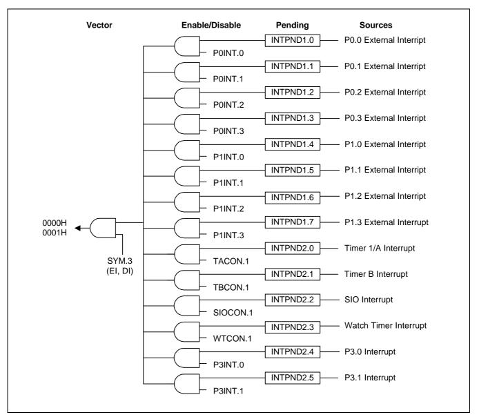
Figure 5-3. S3C9228/P9228 Interrupt Structure
