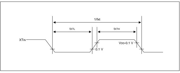
Figure 16-7. Clock Timing Measurement at XT<sub>IN</sub>
