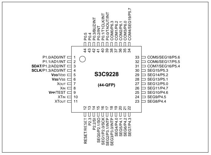
Figure 18-1. S3P9228 44-QFP Pin Assignments
