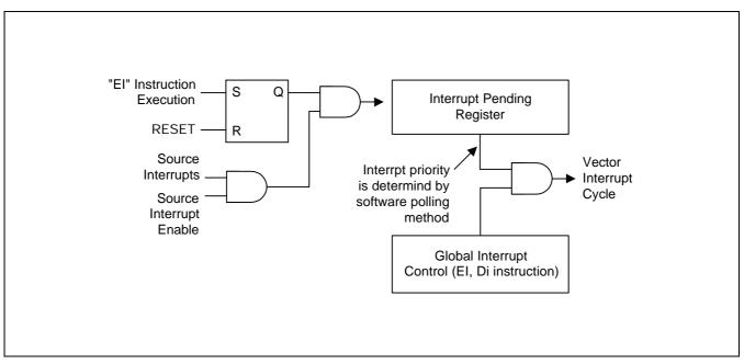
Figure 5-2. Interrupt Function Diagram
