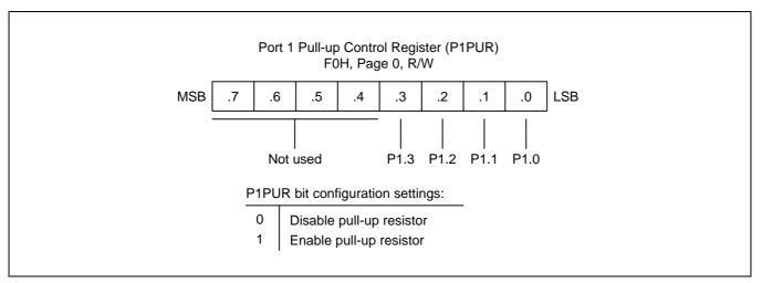
Figure 9-11. Port 1 Pull-up Control Register (P1PUR)
