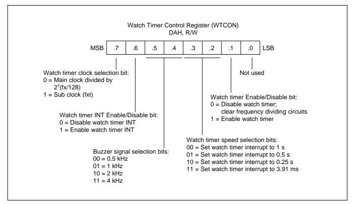
Figure 12-1. Watch Timer Control Register (WTCON)
