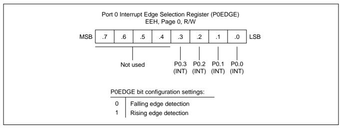
Figure 9-5. Port 0 Interrupt Edge Selection Register (P0EDGE)
