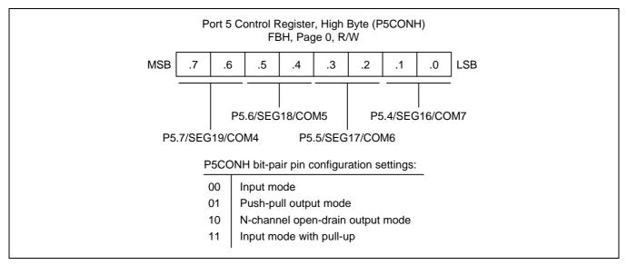
Figure 9-21. Port 5 High-Byte Control Register (P5CONH)
