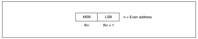
Figure 2-3. 16-Bit Register Pairs
