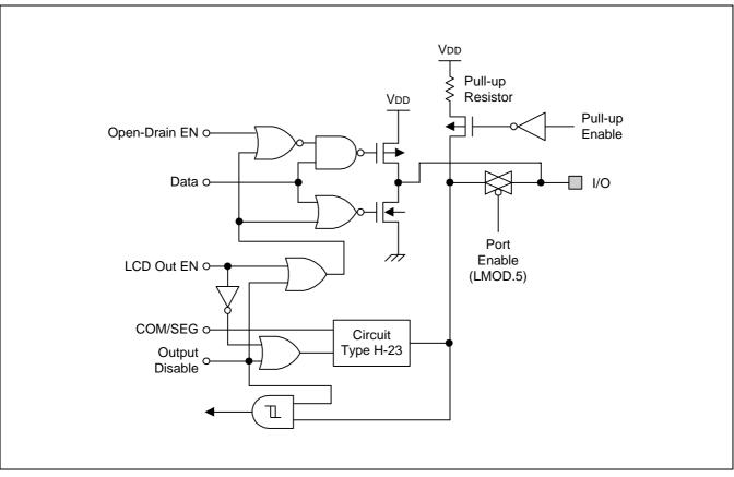
Figure 1-12. Pin Circuit Type H-32B
