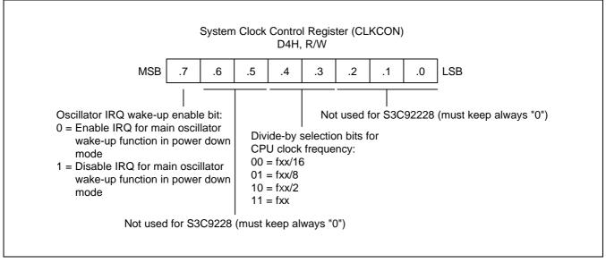
Figure 7-7. System Clock Control Register (CLKCON)
