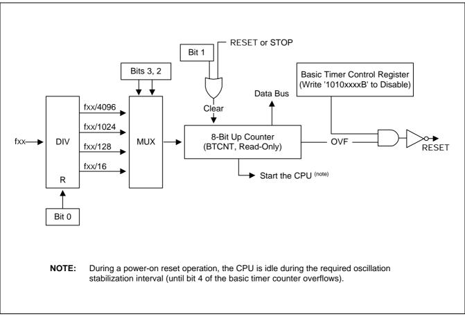
Figure 10-2. Basic Timer Block Diagram
