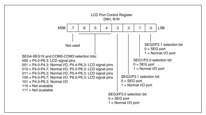
Figure 13-5. LCD Port Control Register
