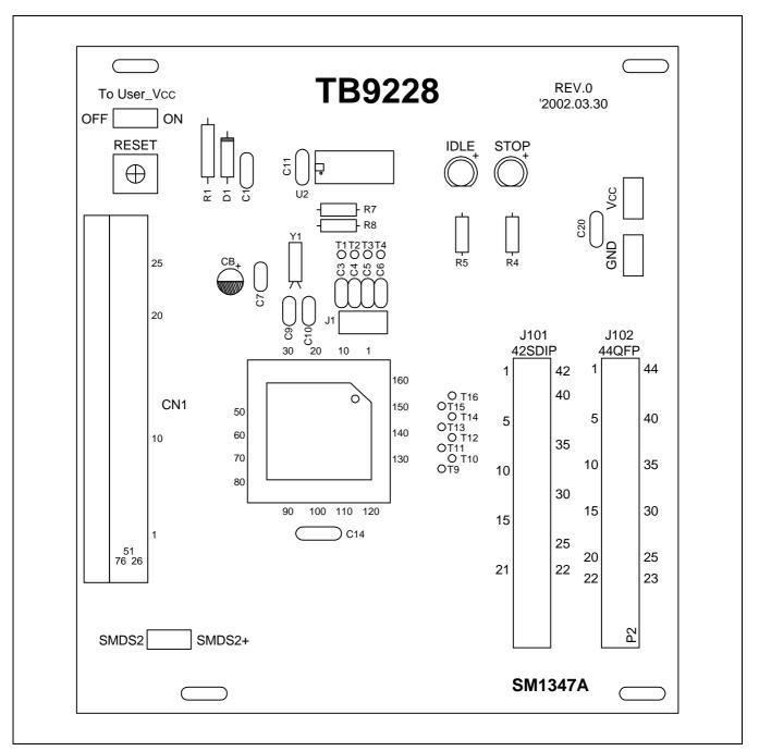
Figure 19-2. TB9228 Target Board Configuration
