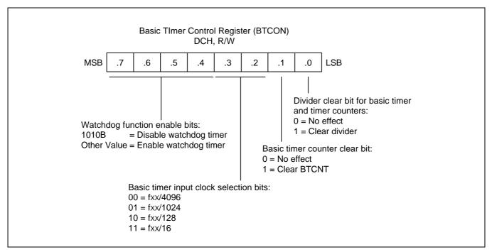
Figure 10-1. Basic Timer Control Register (BTCON)
