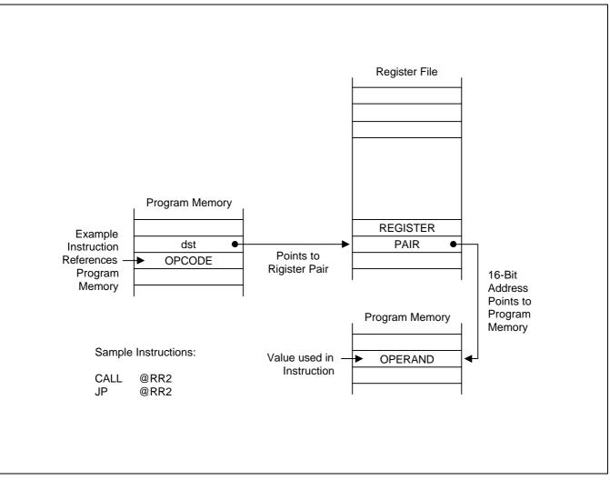
Figure 3-4. Indirect Register Addressing to Program Memory
