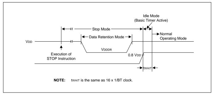
Figure 16-1. Stop Mode Release Timing When Initiated by an External Interrupt
