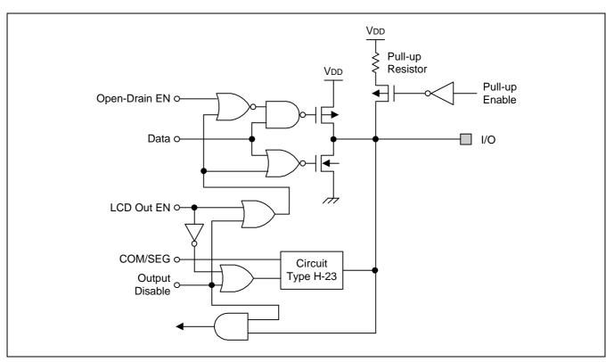
Figure 1-10. Pin Circuit Type H-32
