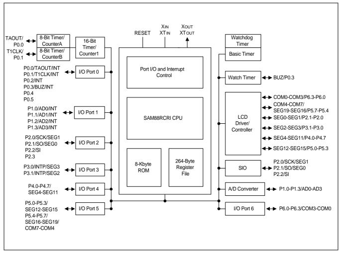
Figure 1-1. Block Diagram
