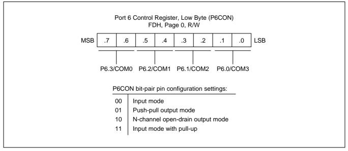
Figure 9-23. Port 6 Control Register (P6CON)
