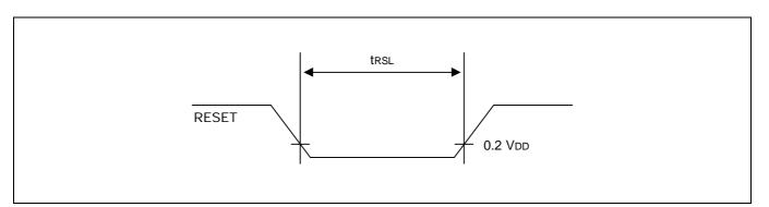
Figure 16-4. Input Timing for RESET
