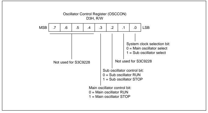
Figure 7-8. Oscillator Control Register (OSCCON)
