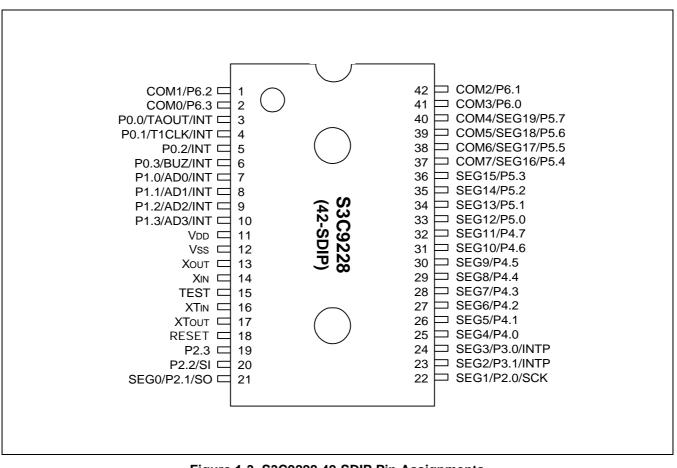
Figure 1-3. S3C9228 42-SDIP Pin Assignments
