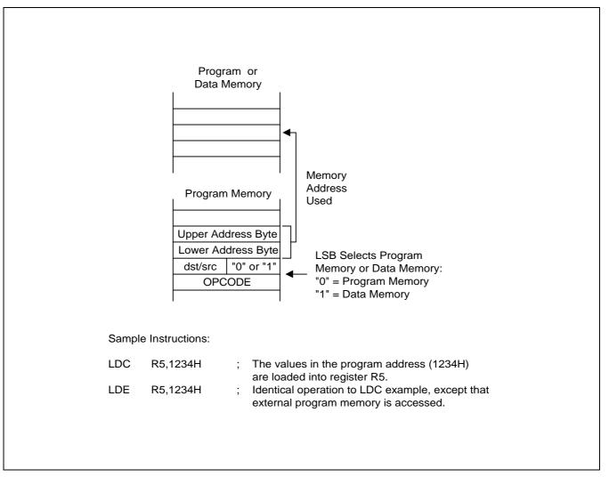
Figure 3-10. Direct Addressing for Load Instructions
