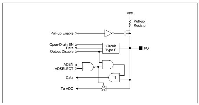
Figure 1-8. Pin Circuit Type F-16A
