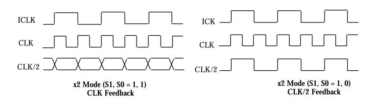
Using CLK as the feedback will always result in synchronized rising edges between ICLK and CLK. But the CLK/2 could be a falling edge compared with ICLK. Therefore, wherever possible, we recommend the use of CLK/2 feedback. This will synchronize the rising edges of all 3 clocks.
