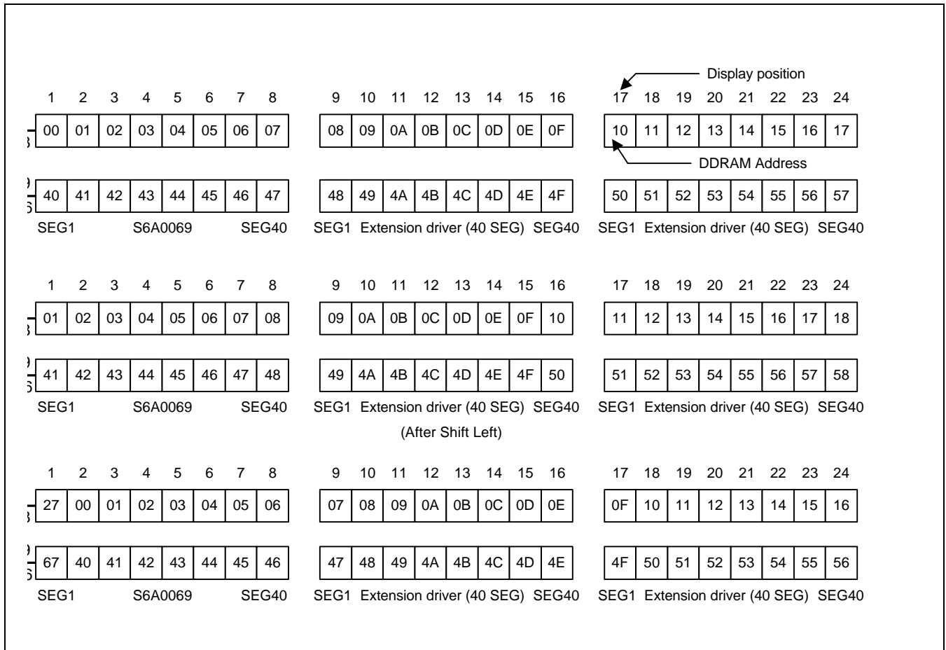
Figure 3. 2-line x 24 Character Display with 40 Segment Extension Driver
