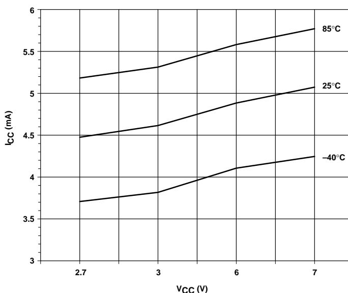
Figure 4. Supply Current vs Supply Voltage and Temperature With No Load
