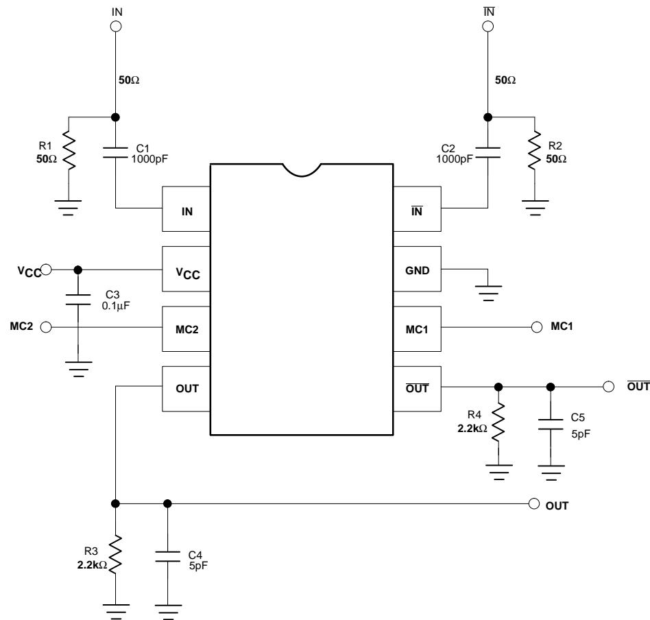
Figure 1. SA702 Test Circuit
