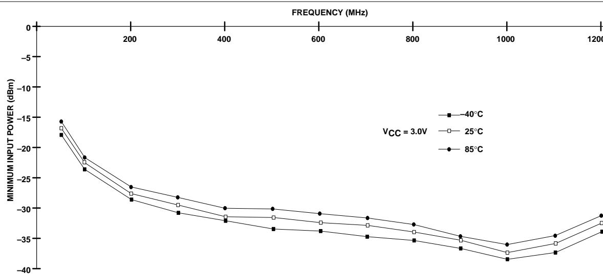
Figure 2. Minimum Input Power vs Frequency and Temperature
