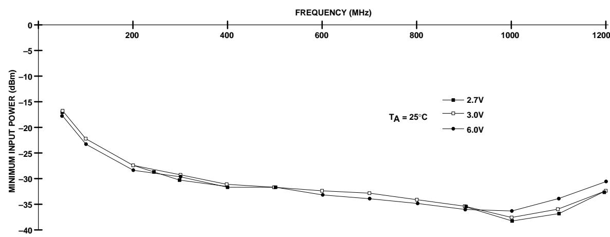
Figure 3. Minimum Input Power vs Frequency and  $V_{CC}$
