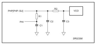
Figure 7. Typical passive 3-pole loop filter.
