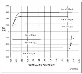
Figure 15. PHP charge pump output vs. Iset  $(CP = 10_3x, V_{DD} = 3.0 \text{ V}, Temp = 25 ^{\circ}\text{C})$
