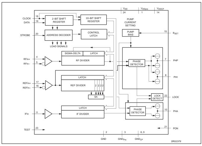
Figure 2. HBCC24 Block Diagram
