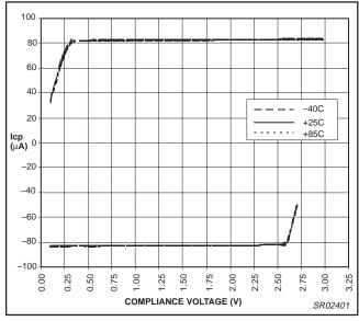
Figure 24. PHA charge pump output vs. temperature (CP = 11\_0.5x,  $V_{DD}$  = 3.0 V, Iset = 163  $\mu$ A)
