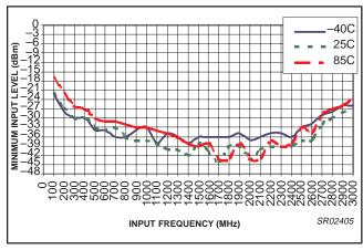
Figure 28. RF (main) divider input sensitivity vs. frequency and temperature ( $V_{CC}$  = 3.0 V, Iset = 164  $\mu$ A, N = 509)
