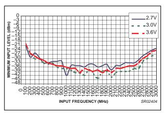
Figure 27. RF (main) divider input sensitivity vs. frequency and supply voltage (Temp = 25  $^{\circ}$ C, lset = 164  $\mu$ A, N = 509)
