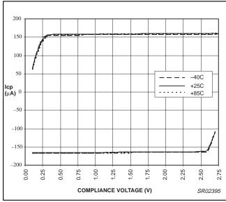
Figure 18. PHP charge pump output vs. temperature (CP = 11\_1x,  $V_{DD}$  = 3.0 V, lset = 163  $\mu$ A)
