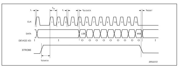
Figure 9. Serial bus "Read" timing diagram.
