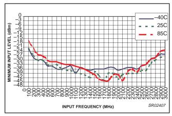
Figure 30. RF (main) fractional divider input sensitivity vs. frequency and temperature (V<sub>CC</sub> = 3.0 V, Iset = 164  $\mu$ A, N = 509.5)
