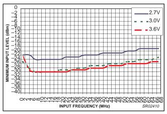
Figure 33. Reference divider input sensitivity vs. frequency and supply voltage (Temp = 25  $^{\circ}$ C, lset = 164  $\mu$ A, divider ratio = 1023)
