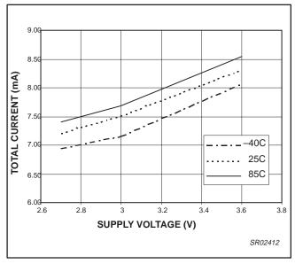
Figure 35. Total supply current vs. temperature (Iset =  $163 \mu A$  Fcomp =  $20 \mu J$ )
