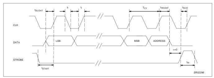
Figure 8. Serial bus "Write" timing diagram.
