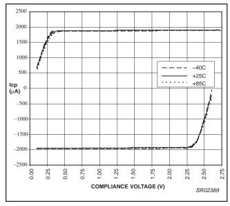
Figure 12. PHI\_SU charge pump output vs. temperature (CP = 01\_12x,  $V_{DD}$  = 3.0 V, Iset = 163  $\mu$ A)
