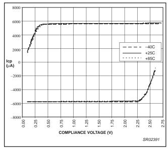
Figure 14. PHI\_SU charge pump output vs. temperature (CP =  $00_36x$ ,  $V_{DD}$  = 3.0 V, Iset =  $163 \mu A$ )
