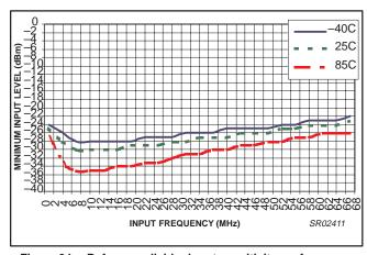
Figure 34. Reference divider input sensitivity vs. frequency and temperature ( $V_{CC}=3.0$  V, lset = 164  $\mu$ A, divider ratio = 1023)
