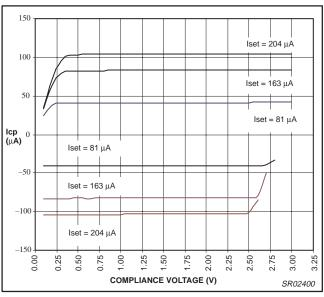
Figure 23. PHA charge pump output vs. lset (CP =  $11_0.5x$ ,  $V_{DD} = 3.0 V$ , Temp =  $25 \,^{\circ}C$ )
