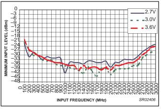
Figure 29. RF (main) fractional divider input sensitivity vs. frequency and supply voltage (Temp = 25  $^{\circ}$ C, lset = 164  $\mu$ A, N = 509.5)
