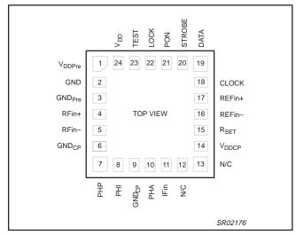
Figure 1. HBCC24 pin configuration.
