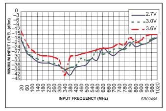
Figure 31. IF (aux) divider input sensitivity vs. frequency and supply voltage (Temp = 25  $^{\circ}$ C, lset = 164  $\mu$ A, divider ratio = 16383)
