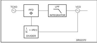
Figure 4. PLL block diagram.
