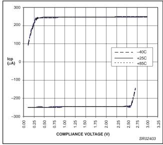
Figure 26. PHA charge pump output vs. temperature (CP = 10\_1.5x,  $V_{DD}$  = 3.0 V, Iset = 163  $\mu$ A)
