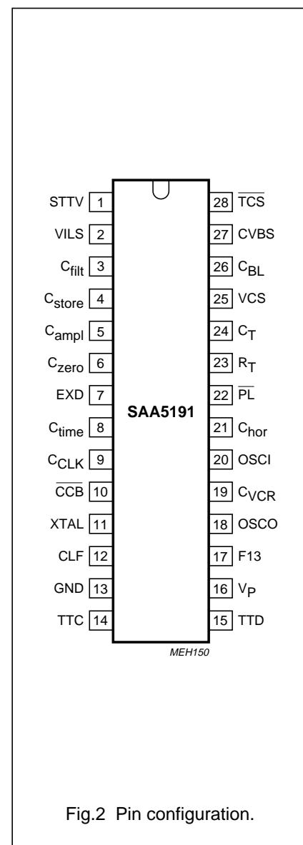
Fig.2 Pin configuration.
