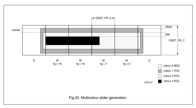
When putting together a slider with multiple characters (see Fig.20), a slider always consists of three basic parts: a start part (S), a middle part (M) with different fill grades (fg) and an ending part (E).
