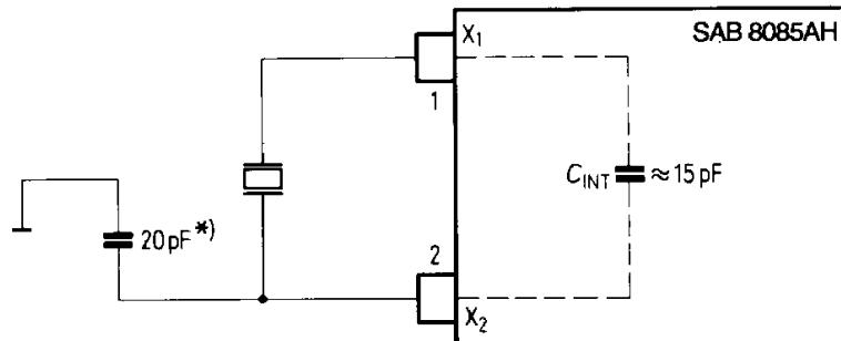
\*) 20 pF Capacitors required for Crystal Frequency  $\leq 4$  MHz only.
