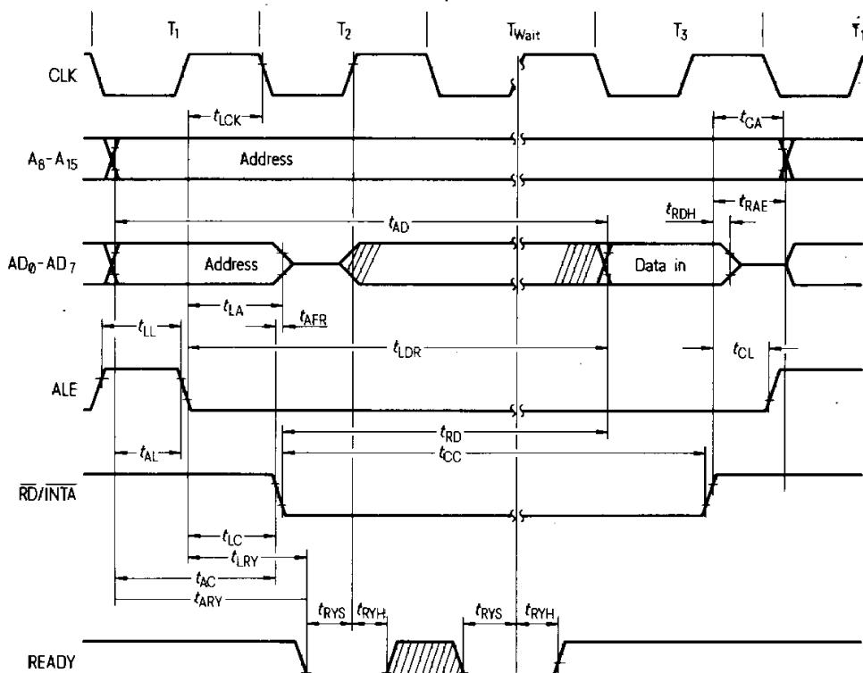
READY must remain stable during setup and hold times.
