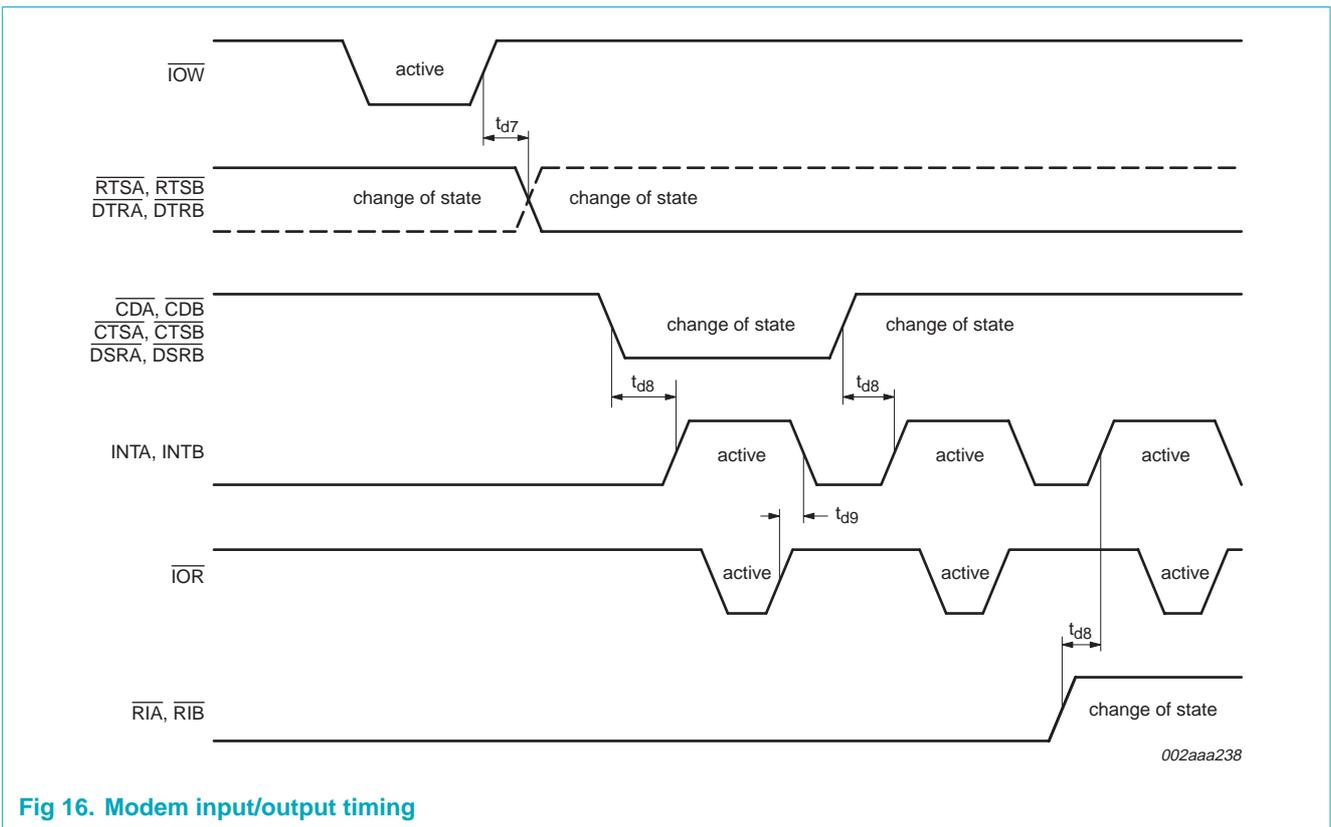
Fig 16. Modem input/output timing
