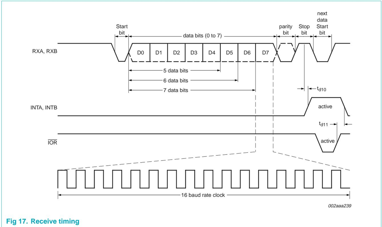
Fig 17. Receive timing
