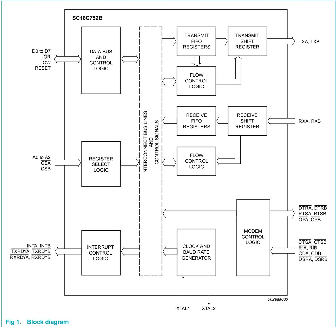
Fig 1. Block diagram
