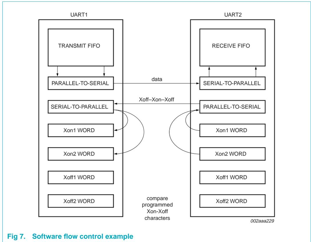
Fig 7. Software flow control example
