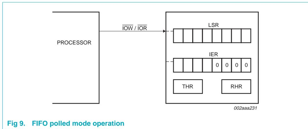
Fig 9. FIFO polled mode operation
