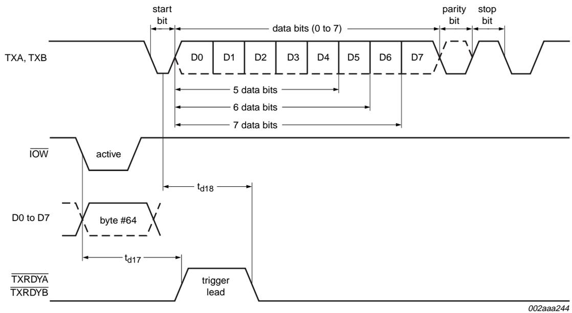
Fig 22. Transmit ready timing in FIFO mode
