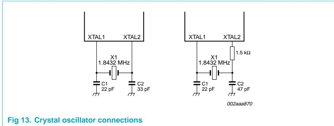
Fig 13. Crystal oscillator connections
