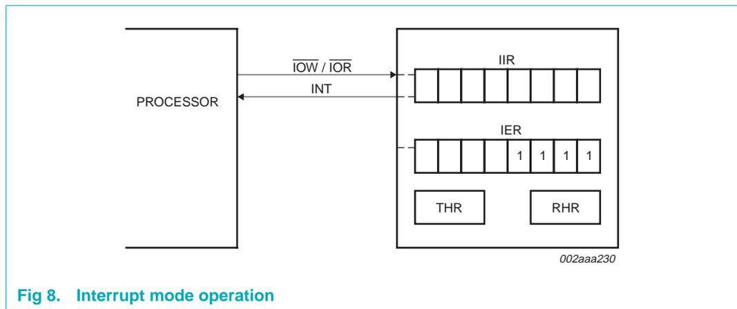
Fig 8. Interrupt mode operation
