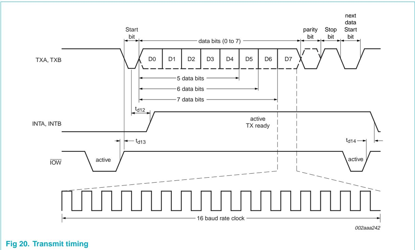
Fig 20. Transmit timing
