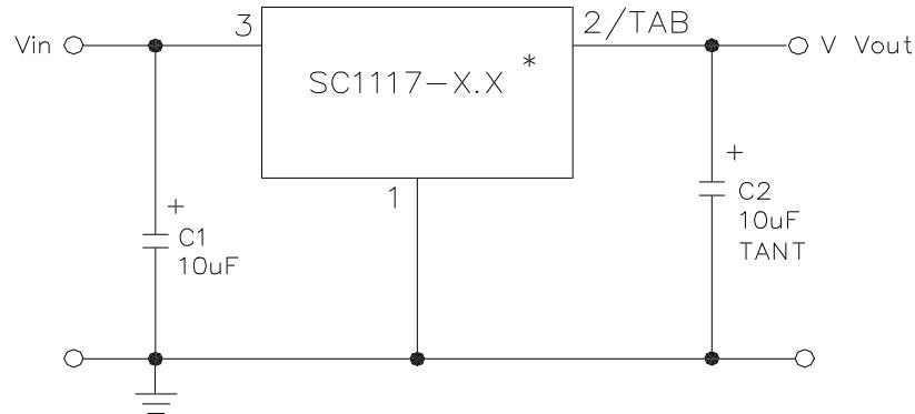
(1) C1 NEEDED IF DEVICE IS FAR FROM FILTER CAPACITORS.
