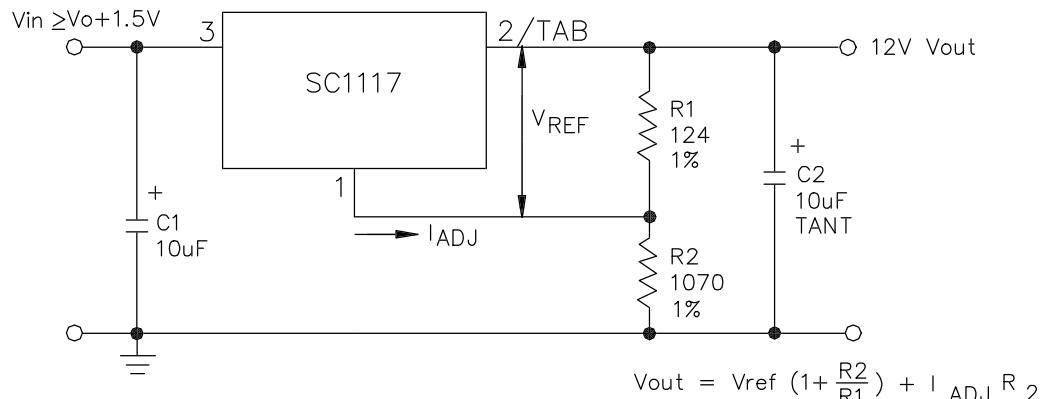
$$V_{out} = V_{ref} \left(1 + \frac{R_2}{R_1}\right) + I_{ADJ} R_2$$
