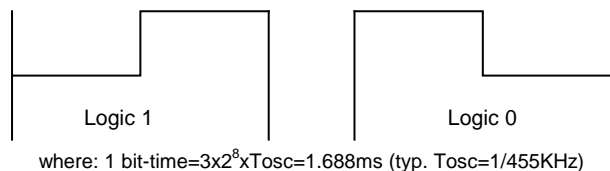
Figure 2: Biphase Code Transmission Technique
