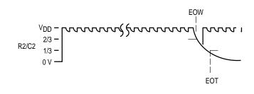
Figure 16. R-C Decay on Pin 10 (R2/C2)
