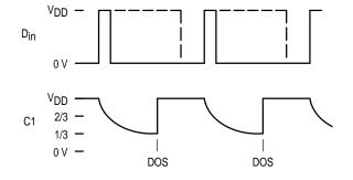
Figure 15. R-C Decay on Pin 7 (C1)
