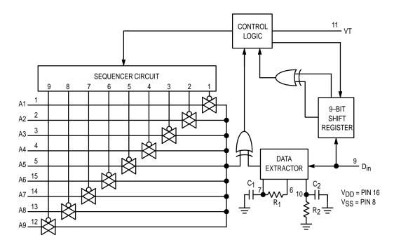
Figure 3. MC145028 Decoder Block Diagram
