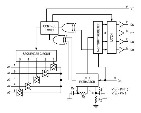
Figure 2. MC145027 Decoder Block Diagram
