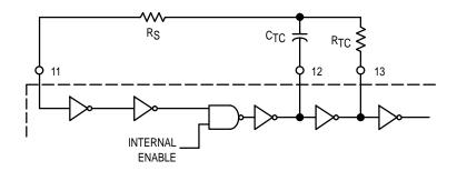
This oscillator operates at a frequency determined by the external RC network; i.e.,
