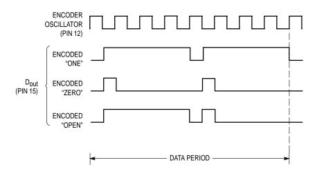
Figure 11. Encoder Data Waveforms
