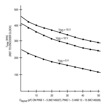
Figure 12. f<sub>max</sub> vs  $C_{layout}$  — Decoders Only
