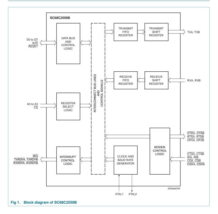
5 V, 3.3 V and 2.5 V dual UART, 5 Mbit/s (max.), with 16-byte FIFOs
