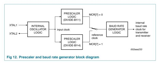
DLL and DLH must be written to in order to program the baud rate. DLL and DLH are the least significant and most significant byte of the baud rate divisor. If DLL and DLH are both zero, the UART is effectively disabled, as no baud clock will be generated.
