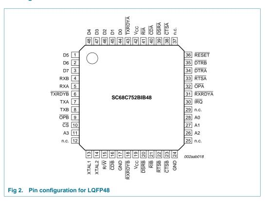
5 V, 3.3 V and 2.5 V dual UART, 5 Mbit/s (max.), with 64-byte FIFOs
