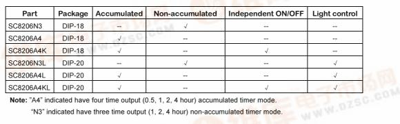
Note: "A4" indicated have four time output (0.5, 1, 2, 4 hour) accumulated timer mode.
