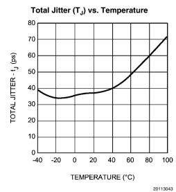
Total Jitter measured at 0V differential while running a PRBS 2<sup>23-1</sup> pattern with a single channel active.  $V_{CC}$  = 3.3V,  $V_{ID}$  = 0.5V,  $V_{CM}$  = 1.2V, 1.5 Gbps data rate, 0% Pre-emphasis
