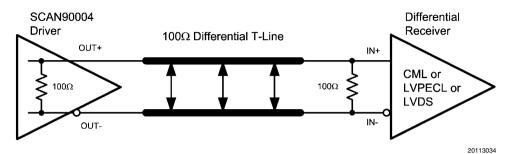
Typical SCAN90004 Output DC-Coupled Interface to an LVDS, CML or LVPECL Receiver
