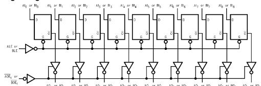
$AO_0$  or  $BO_0$   $AO_1$  or  $BO_1$   $AO_2$  or  $BO_2$   $AO_3$  or  $BO_3$   $AO_4$  or  $BO_4$   $AO_5$  or  $BO_5$   $AO_6$  or  $BO_6$   $AO_7$  or  $BO_7$  Please note that this diagram is provided only for the understanding of logic operations and should not be used to estimate propagation delays.
