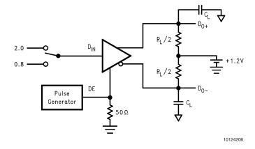
FIGURE 4. Driver TRI-STATE Delay Test Circuit
