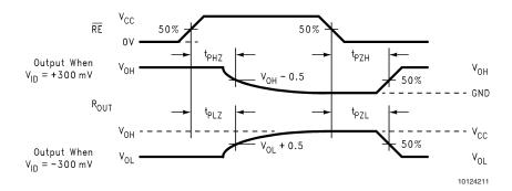
FIGURE 9. Receiver TRI-STATE Delay Waveforms
