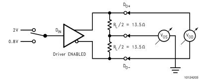
FIGURE 1. Differential Driver DC Test Circuit
