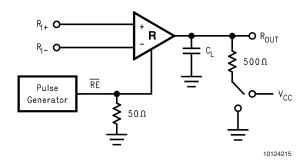
FIGURE 8. Receiver TRI-STATE Delay Test Circuit
