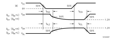
FIGURE 5. Driver TRI-STATE Delay Waveforms
