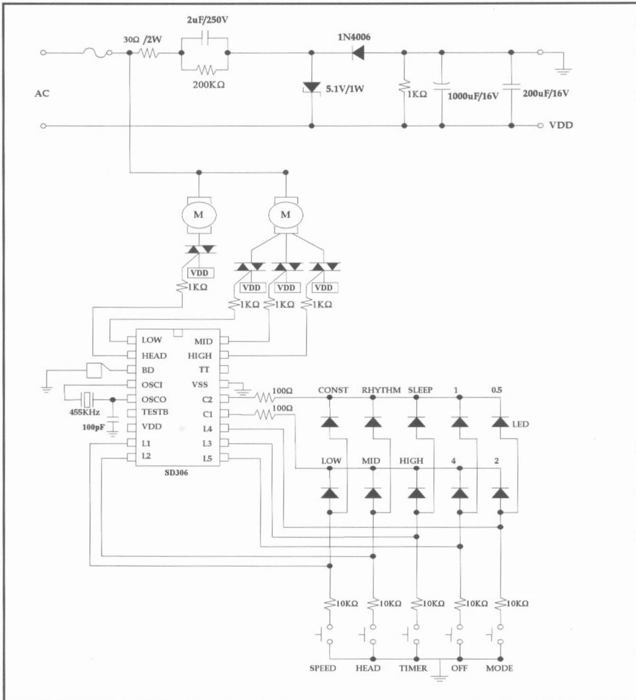
**Fig 1. SD306 Typical Application Circuit.**
