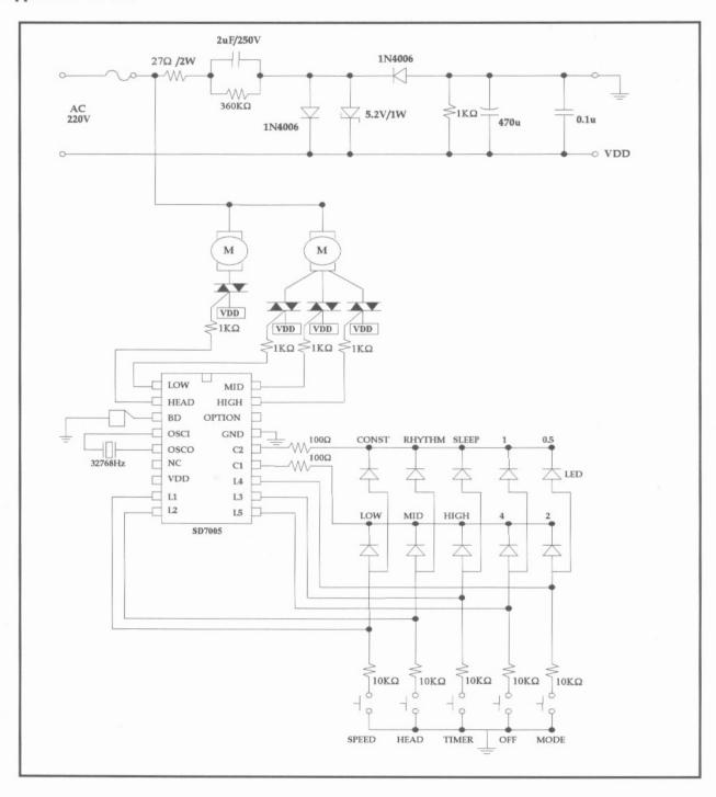
Fig 1. SD7005 Typical Application Circuit.
